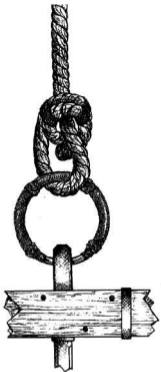
C13 METHOD OF ATTACHING THE ANCHOR CABLE TO THE ANCHOR (no scale)
