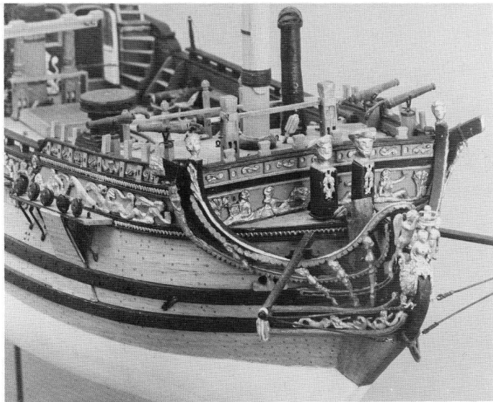
10. Bow view, showing details of the figurehead group, knightheads and decoration.
