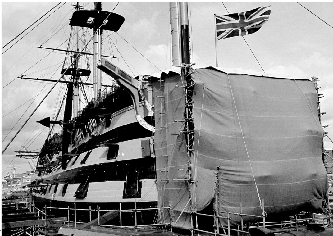
Victory's bowsprit, figurehead and part of her beakhead under restoration in 1983. Jonathan Eastland/Ajax
