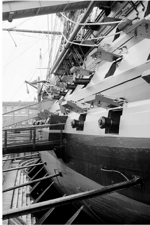
Nelson's flagship seen from the port quarter bristling with cannon. The effect of the tumblehome to the sides of the ship is clearly seen. Jonathan Eastland/Ajax
