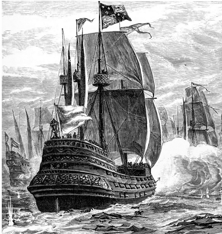
A nineteenth century engraving of how an Elizabethan naval ship of 1588 might have looked as it harassed the Spanish Armada; four masted, long, low and race built according to the philosophy of Sir John Hawkins. The letters E-R are carved into the stern of this fifty gun monster. Ajax Vintage Picture Library
