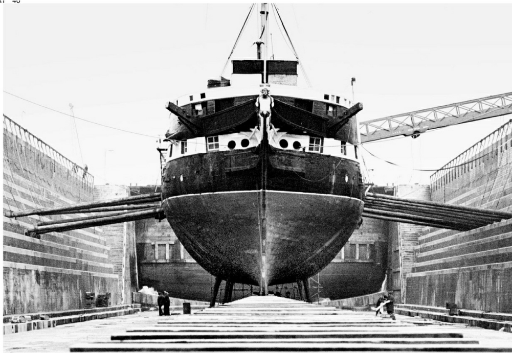
The training ship Foudroyant in Southampton's Number 5 dry dock in the 1970s. She is docked in the traditional way, with wooden props. The elegant underbody shape of fighting sailing ships of the eighteenth and early nineteenth century is clearly seen. Jonathan Eastland/Ajax
