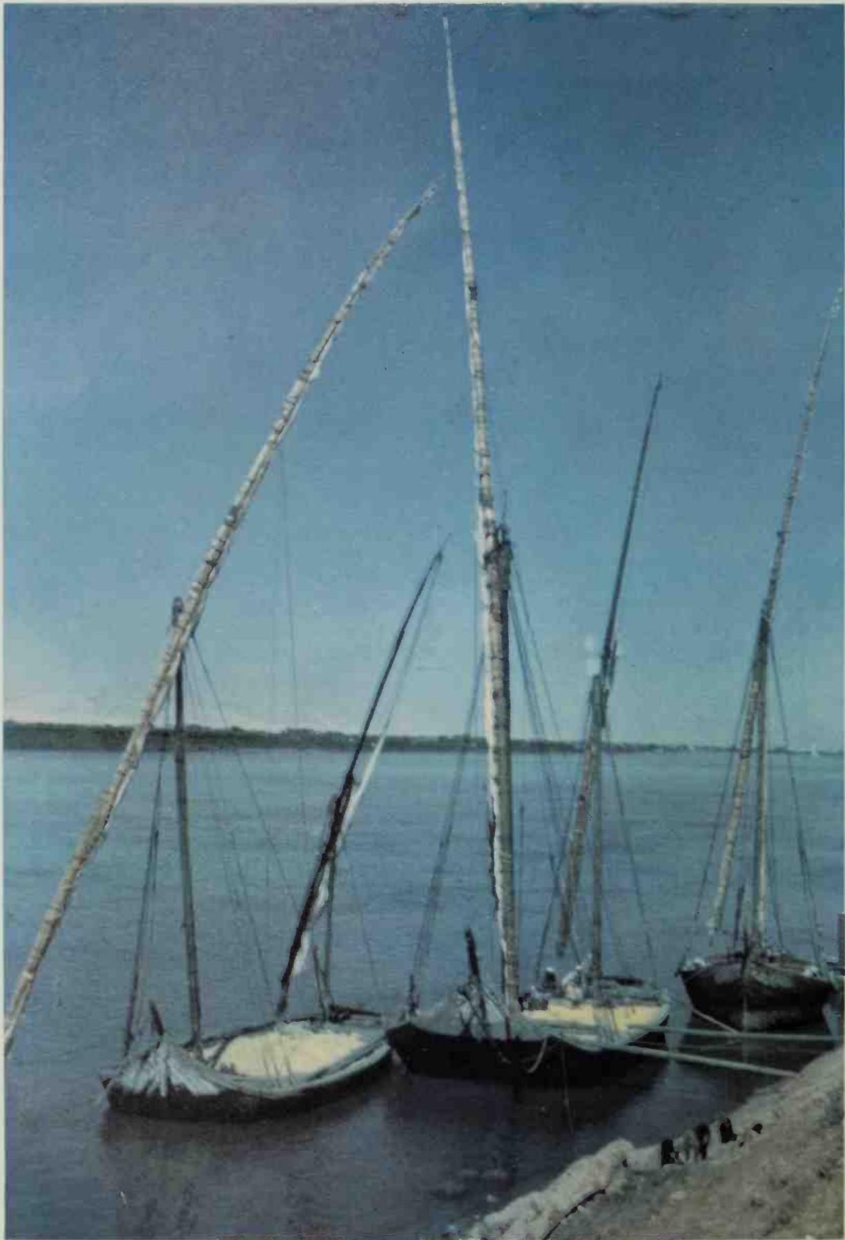
234, 234A. A group of ghayassabs , the workhorses of the lower Nile. They are flat-bottomed. The low sterns and the high bows, decked up to the stem at a steep angle, are typical. On an eighty-foot ghayassab , the main yard can run fully eighty-four feet long and the mizzen fifty feet. See page 198.
