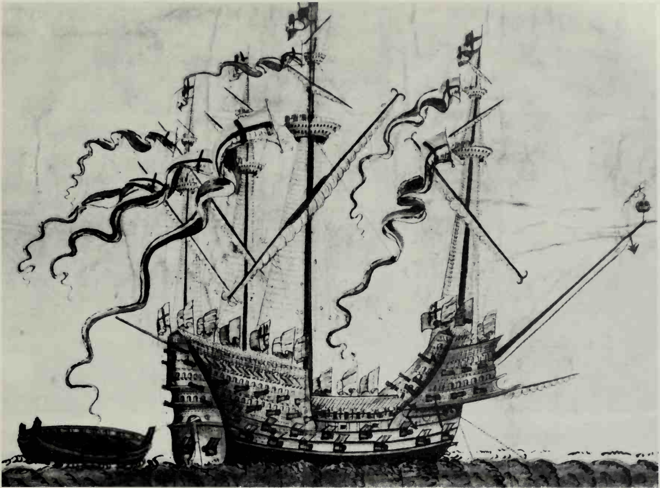
116. The Henry Grâce à Dieu as rebuilt in 1545. In this contemporary drawing the proportions, particularly the height, are exaggerated, but the distinctive features are clear: rounded hull with its bulging carrack prow, solid sterncastle, and square stern; the rig with yards for twelve sails; the guns, particularly the main battery—two rows firing through ports in the side.
