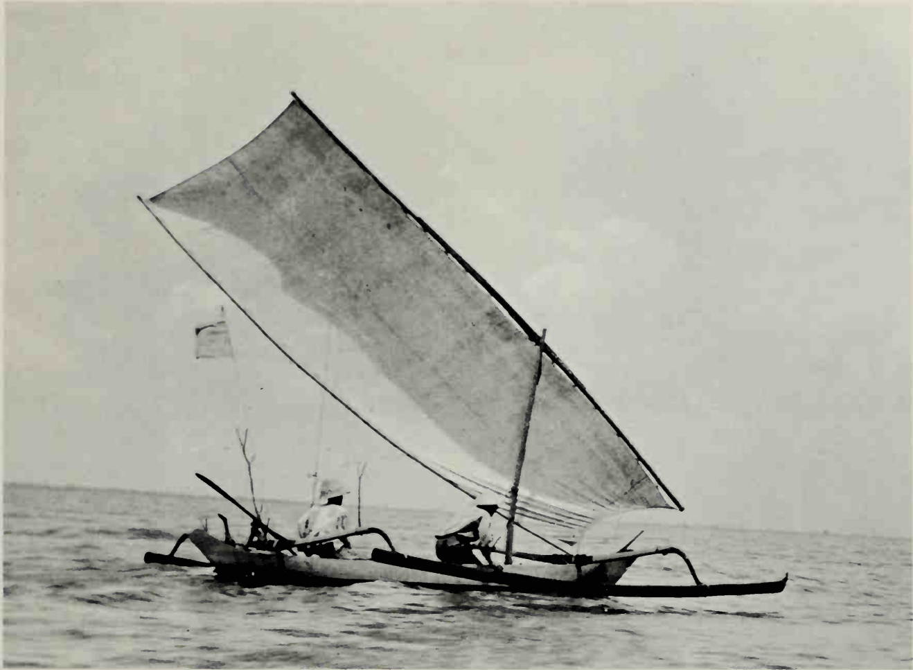
249. A double-outrigger canoe of Java with an Indonesian balance lug.
