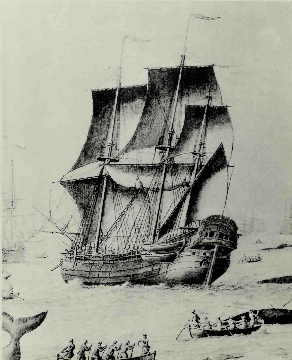
176. The Vergulde Walvis ("Golden Whale"), a Dutch whaler of the early seventeenth century at work in northern waters. The vessel has a sturdy, roomy hull, and her rig is the basic six-sail type plus a mizzen topsail and that hallmark of the seventeenth century, the spritsail topsail.
