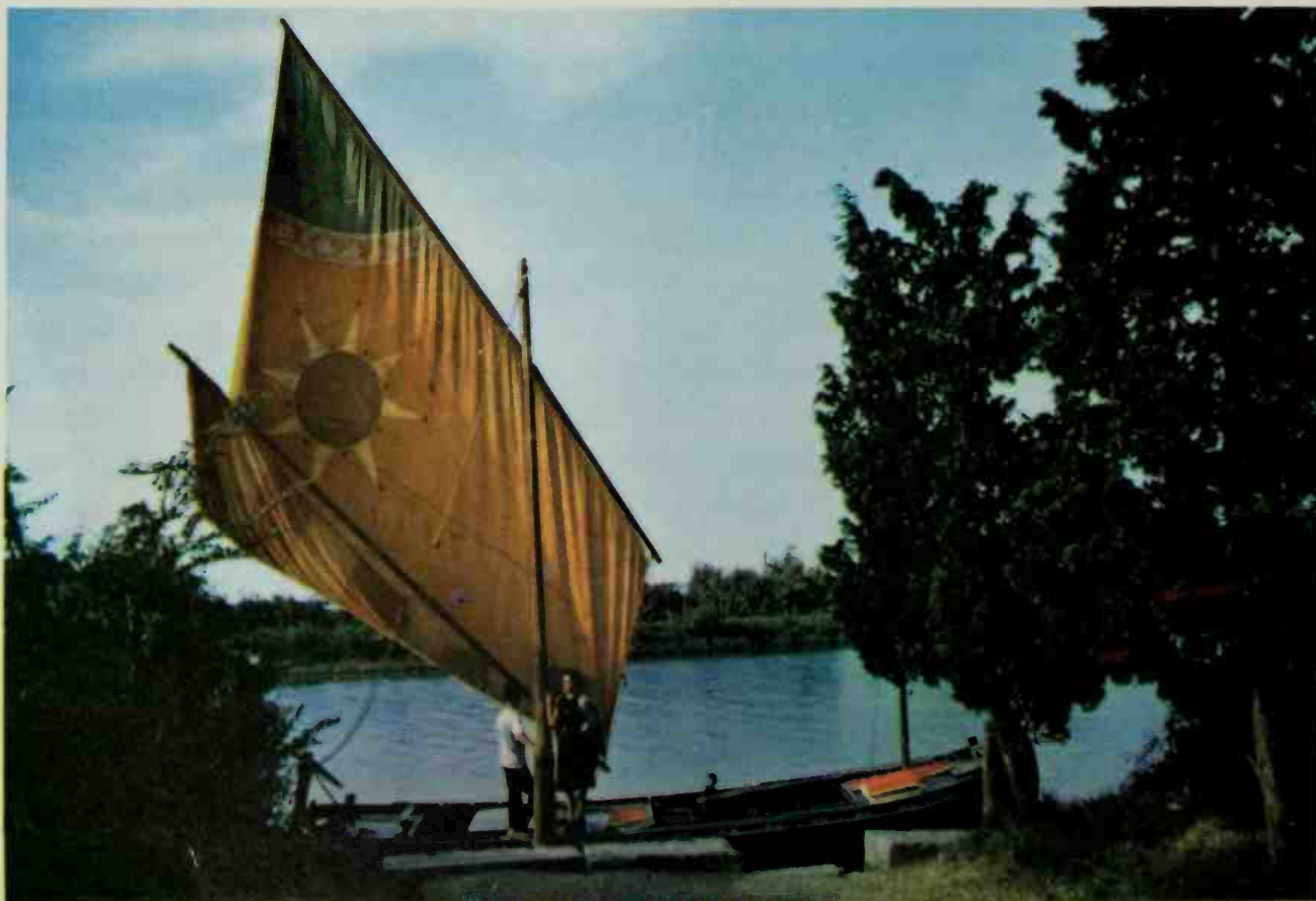
229. The bragozzo , the slender, flat-bottomed craft used on the lagoons about Venice. The flamboyance of the Venetians isn't limited to their art and architecture; it can be seen, too, in the color of their sails. In addition to its ample mainsail, the bragozzo carries a quite small lug foresail. See page 197.
