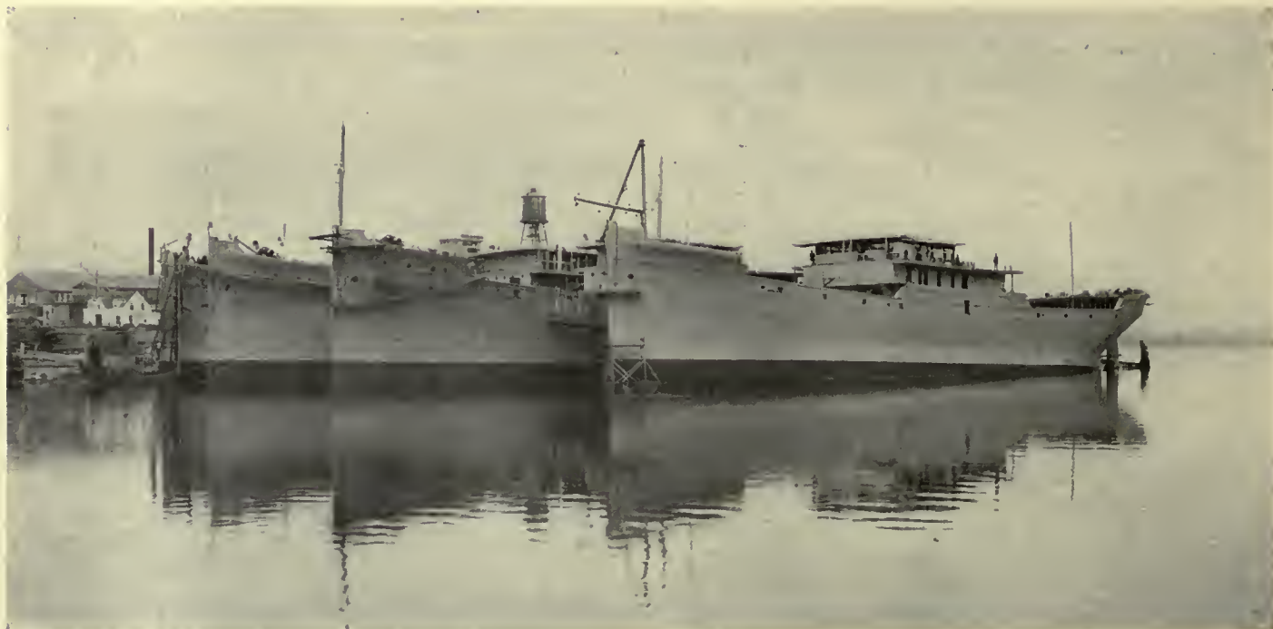
Fig. 143. Chibiabos, Roy H. Beattie, Milton and Haverhill, Four Ships Built by L. H. Shattuck, Inc., at Portsmouth, at the Dock Fitting Out With Rigging, Joiner Work, Etc.
