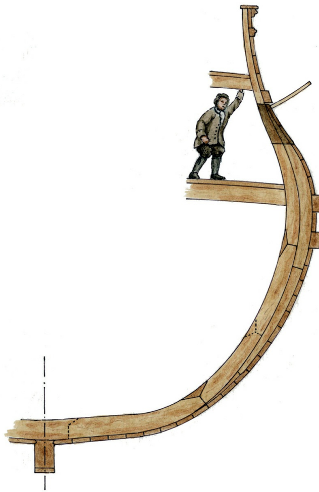
The same ship showing how the extra breadth may have been achieved by furring the frames. Author.
