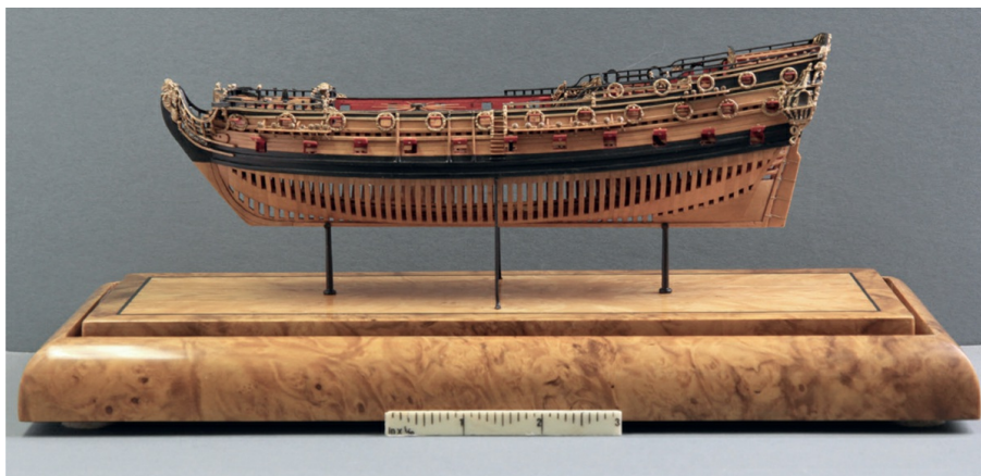
The bow of the model of the Mordaunt. Note the difference between the van de Velde drawing and the model in terms of the position of the channel wale in relation to the forward upper-deck gunport. Photograph by Author, by kind permission of the National Maritime Museum.
