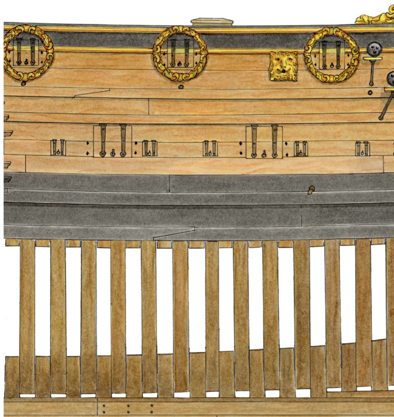
Nearly all models were made with this simplified frame arrangement. The three futtocks on each side used in real ships have been replaced by a single futtock. The middle futtock that normally sits between the floor and the toptimber is eliminated and the lower and upper futtocks that overlap them are merged into one. The heel of the toptimber is just visible below the main wale in its correct place. The frames are of constant width as they reach upward in order to simplify the modelmaking. The open frame style was not just easier to make but also very attractive. Author.
