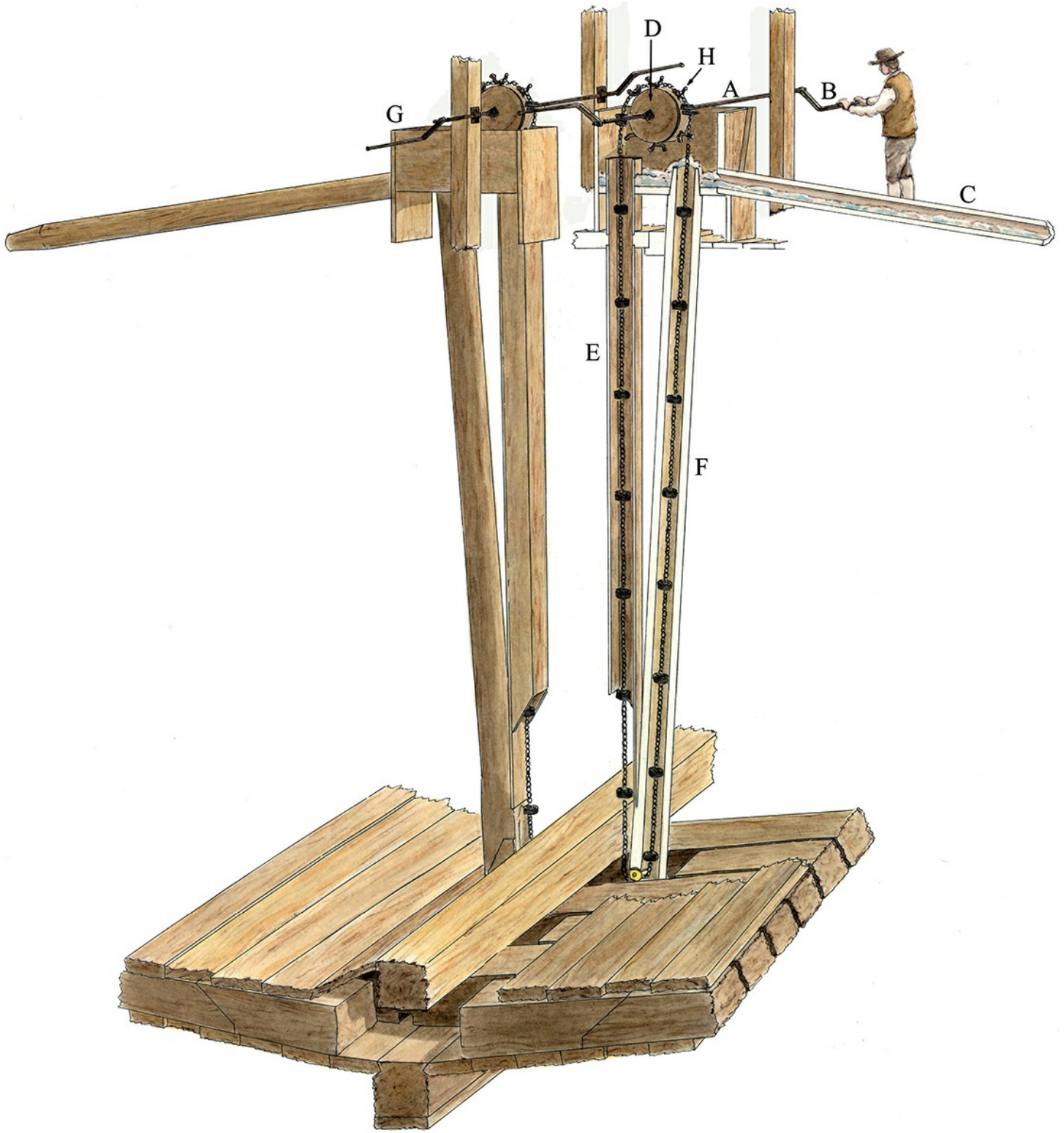
The late-17th-century chain pump. A. Axletree; B. Winch; C. Dale; D. Wheel; E. Case; F. Pump; G. Cistern; H. Sprockets or forks. 229 Author.
