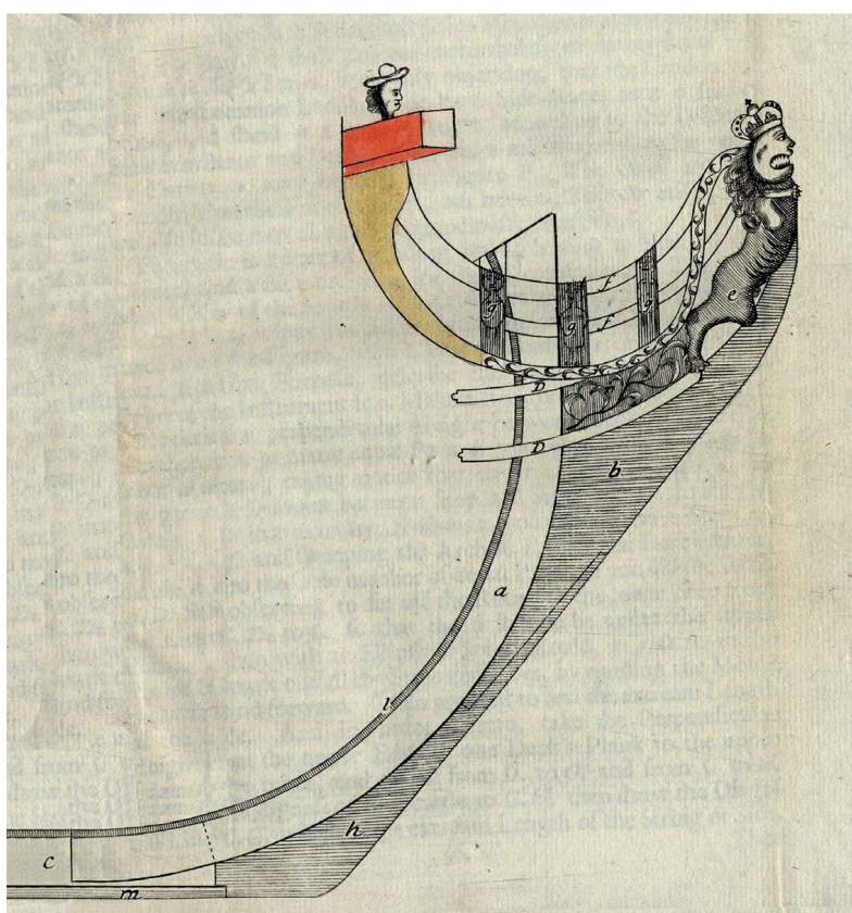
The head of a ship with a circular stem, extracted from William Sutherland's Ship-builders Assistant , 1711, with additions. a. Stem; b. Knee of the head (its foremost part is barbed away and is called the cut-water); c. Forefoot; e. Lyon; d. Checks; f. Rails of the head; g. Brackets; h. Gripe; l. Rabet; m. False keel.
