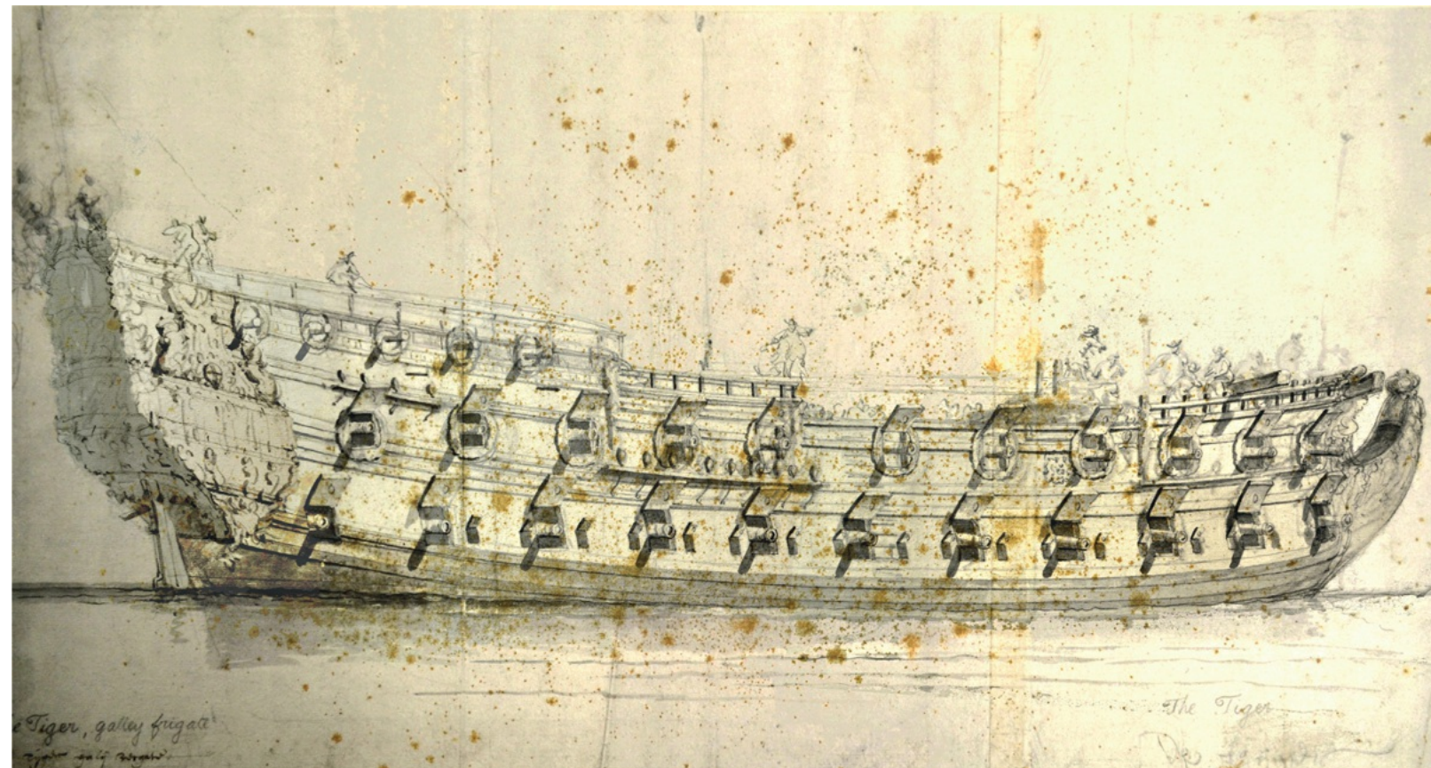
The Tyger , just abaft the starboard beam (Robinson 595). Details of interest are the spare topmast in the waist between the gallows and the forecastle. A flagstaff forward confirms that the drawing was made shortly after the launching at Deptford. The guns would not have been aboard, but have been added by the artist for effect. 11½ x 23 inches, probably a worked-up offset. Portrait of the 'Tiger'. Willem van de Velde, the Elder, 1681? PAG6250; Collection: National Maritime Museum, Greenwich, London.
