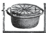
Azimuth and brass box compasses of the type used on the Mordaunt. From A Naval Expositor, Thomas Blanckley, 1750.
