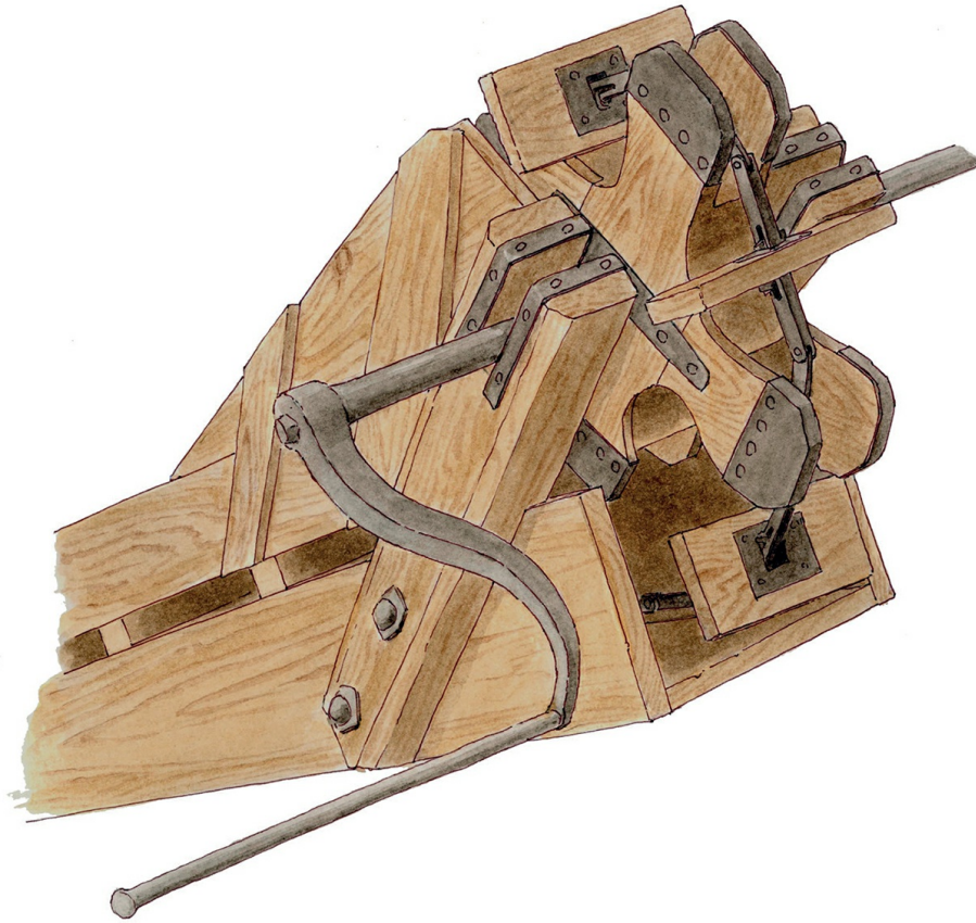
The upper end of the Tudor-period Hampton Court pump. It has been suggested that it was used to remove sewage, but its size and ingenious compact design may indicate a naval connection. The lower (idle) wheel is similar to the upper but not driven. Author.
