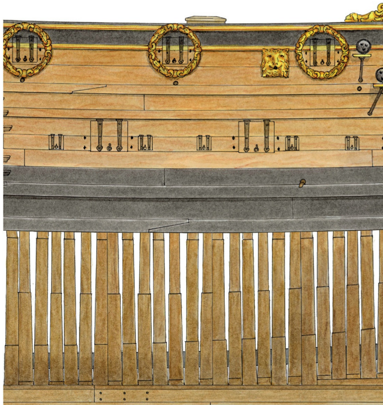
The true arrangement of frames and their component parts as represented in the Tyger of 1681. Almost all other ships, including fourth rates, had the same arrangement. The only exceptions were the largest three-deckers and some small ships. Only one contemporary model with the true late-17th-century fashion of framing is known to exist. 664 Author.
