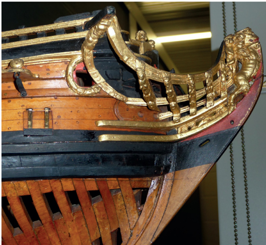
The bow of the model of the Mordaunt. Note the difference between the van de Velde drawing and the model in terms of the position of the channel wale in relation to the forward upper-deck gunport. Photograph by Author, by kind permission of the National Maritime Museum.
