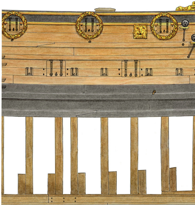
The framing on the model of John Shish's fourth-rate St Albans of 1687 and on the third-rate Boyne of 1692, built by Fisher Harding. They are similar in style to previous Shish models with every other frame eliminated, but even more simplified. They clearly show the reversal of the floor timbers around the midship bend. Author.
