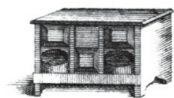
The Mordaunt was built before the introduction of the steering wheel, but the bittacle, shown here, was of the same type used on ships steered with the whipstaff. From A Naval Expositor, Thomas Blanckley, 1750.
