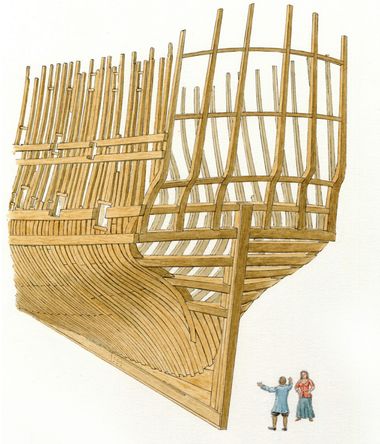
The framing of the stern of the Tyger. The starboard side, furthest away, shows only the frame bends but includes both the full-length transoms and the half transoms attached to the stempost, the inner post and the fashion piece. The half transoms complete an almost solid frame of timber into which to drive the planking treenails. The port side shows all the frame timbers. Note how the main transom and the port helm transom above it are in line with the main wales. The wales and transoms were joined firmly together by large fore and aft knees on the inside of the ship. The two transoms also form the upper and lower sills of the stern gunports. Author.
