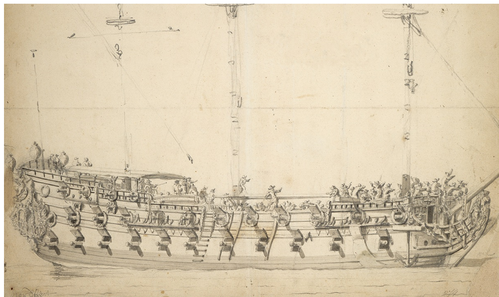
The Mordaunt viewed from slightly before the starboard beam. Compared with the model, a number of additions have been made to equip her for Navy service. These include an anchor lining, lights for the cabins, gallows and side-hung gunport lids in the wake of the main channels. This view also shows the wales near the bow in a different position to those on the model (Robinson 598). Portrait of the 'Mordaunt'. Willem van de Velde, the Elder, 1681? PAH9367; Photo: © National Maritime Museum, Greenwich, London.
