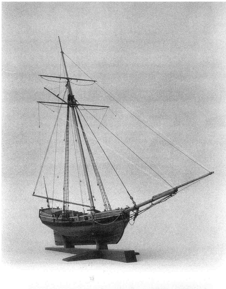
A view of the completed lifts and braces.
