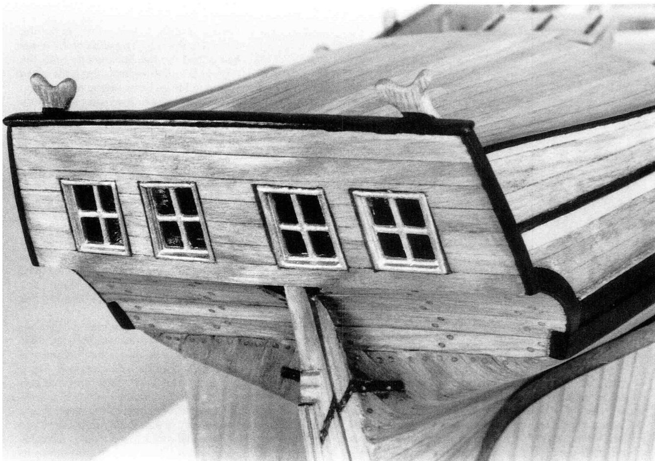
The stern lights installed.
