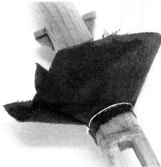
The mast coat wired in place.
