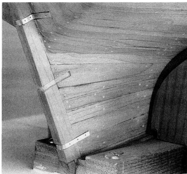
The gudgeons being fitted to the hull (sockets not soldered in place yet).
