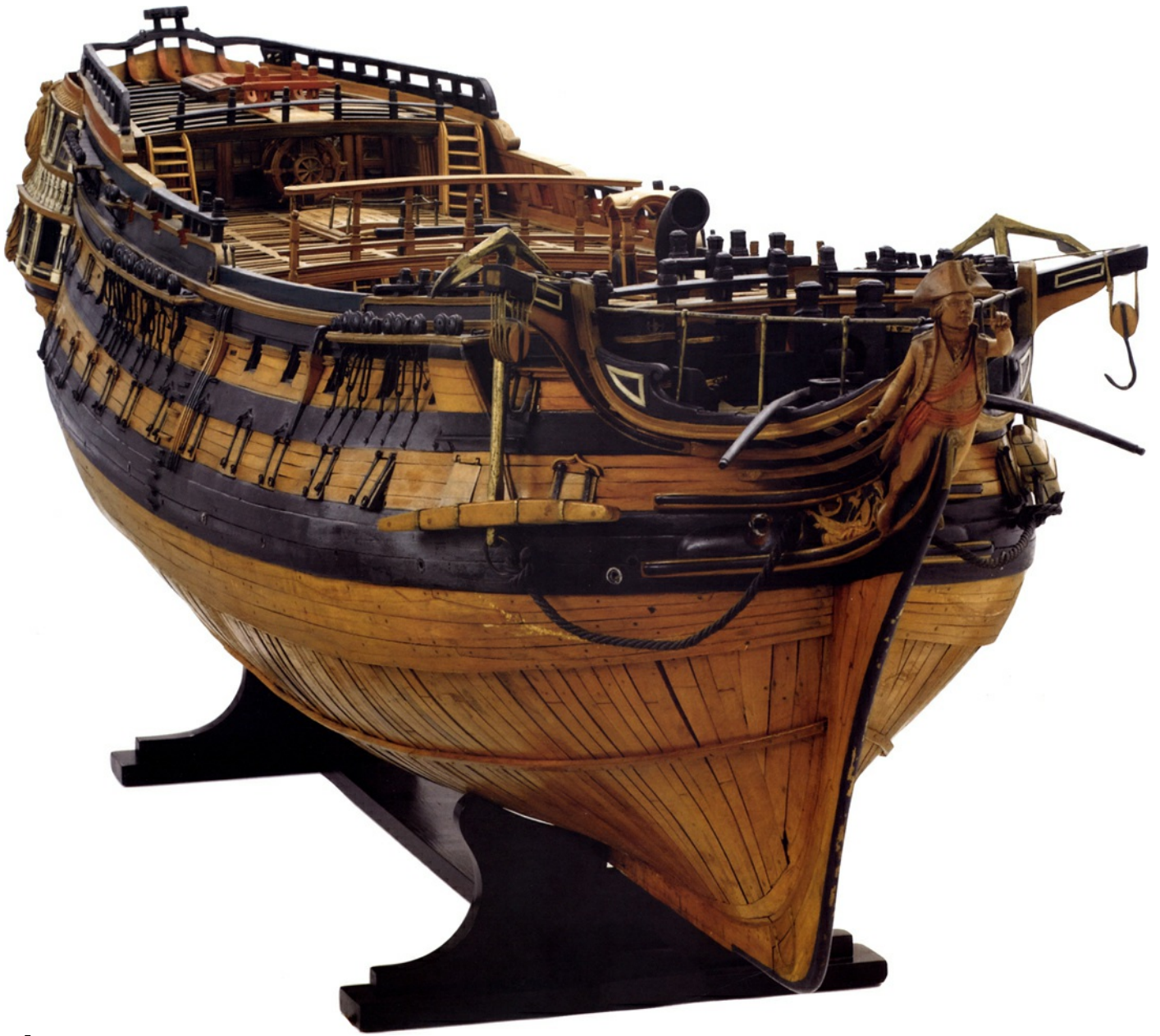
A CONTEMPORARY model at 1/48th scale of a Common Class 74 of about 1790, possibly made for demonstration purposes as the hull is framed and timbered in exact imitation of full-size practice, including wales planked in 'anchor-stock' and 'top and butt' fashion. (F4196-2)
