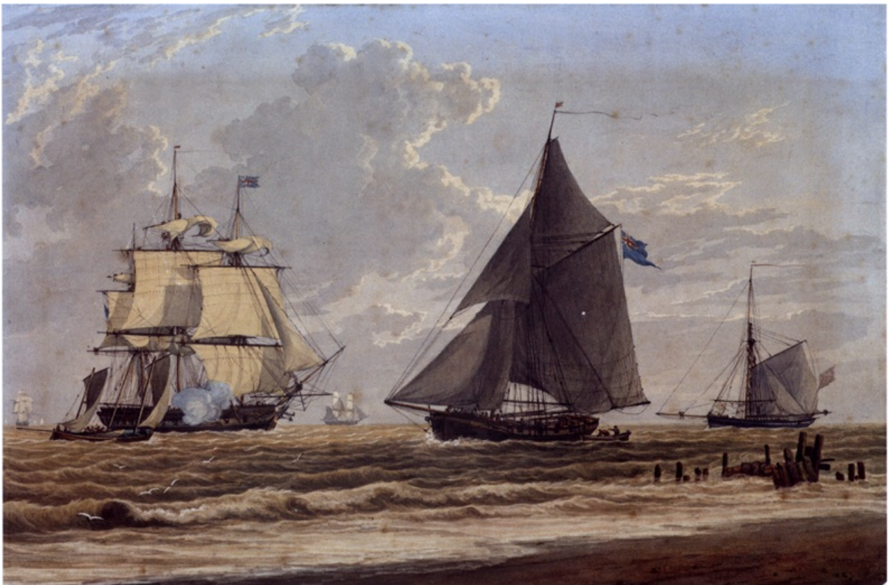
A N anonymous watercolour showing a British frigate and two cutters close inshore. The cutter to the right, shown getting underway, has no obvious gunports but the clinker-built one in the foreground is pierced for twelve guns and may well be naval. The depiction of the craft themselves and the details of their handling shows a seaman-like familiarity with the subject. (PY4080)
