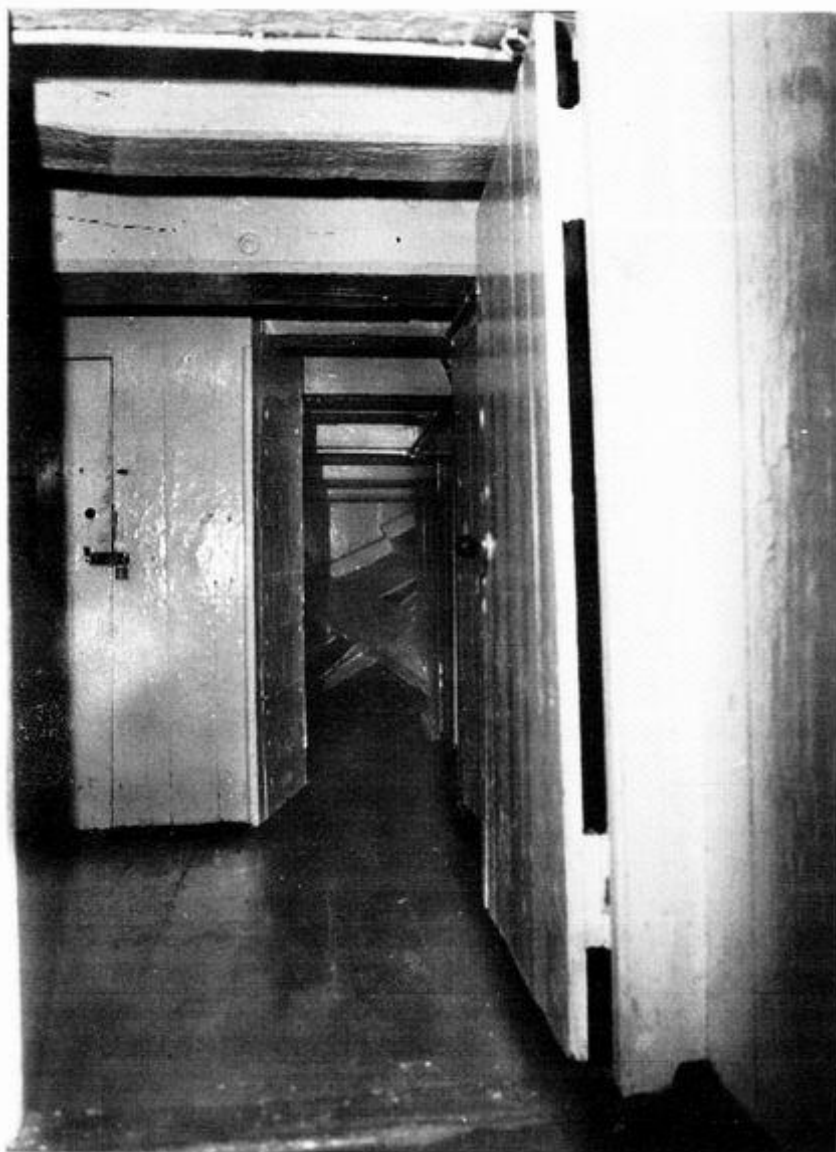
Left: Unicorn. Looking aft into the compartments fitted on the after platform. The passageway on the right which led to the bread room also gave access to the after magazine and its light room.
