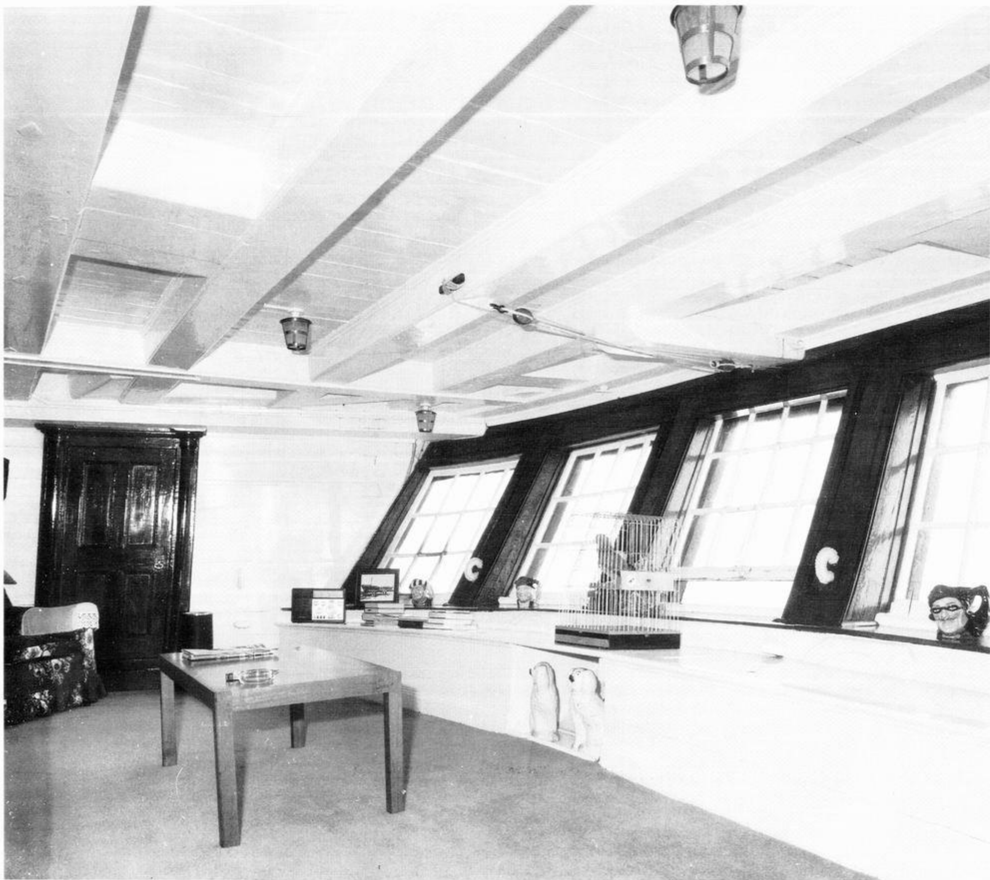
Foudroyant. Captain's day cabin. This view clearly shows the stern counter timbers which are furnished with eyebolts for securing guns. The heavy carlings set in the deckhead are fitted in way of bollards fitted on the deck above. The doorway gives access to the starboard quarter gallery.
