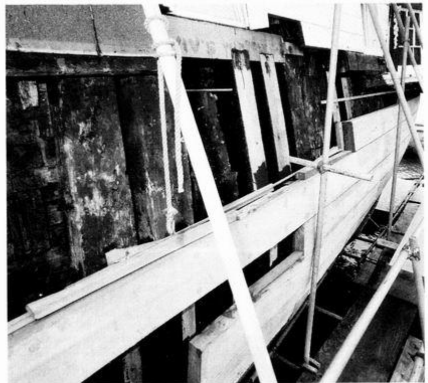
Above: Foudroyant. Port side, aft, showing the framing and gunport sill. The quarter gallery stool and lower finishing have been removed to allow restoration work to be carried out.
