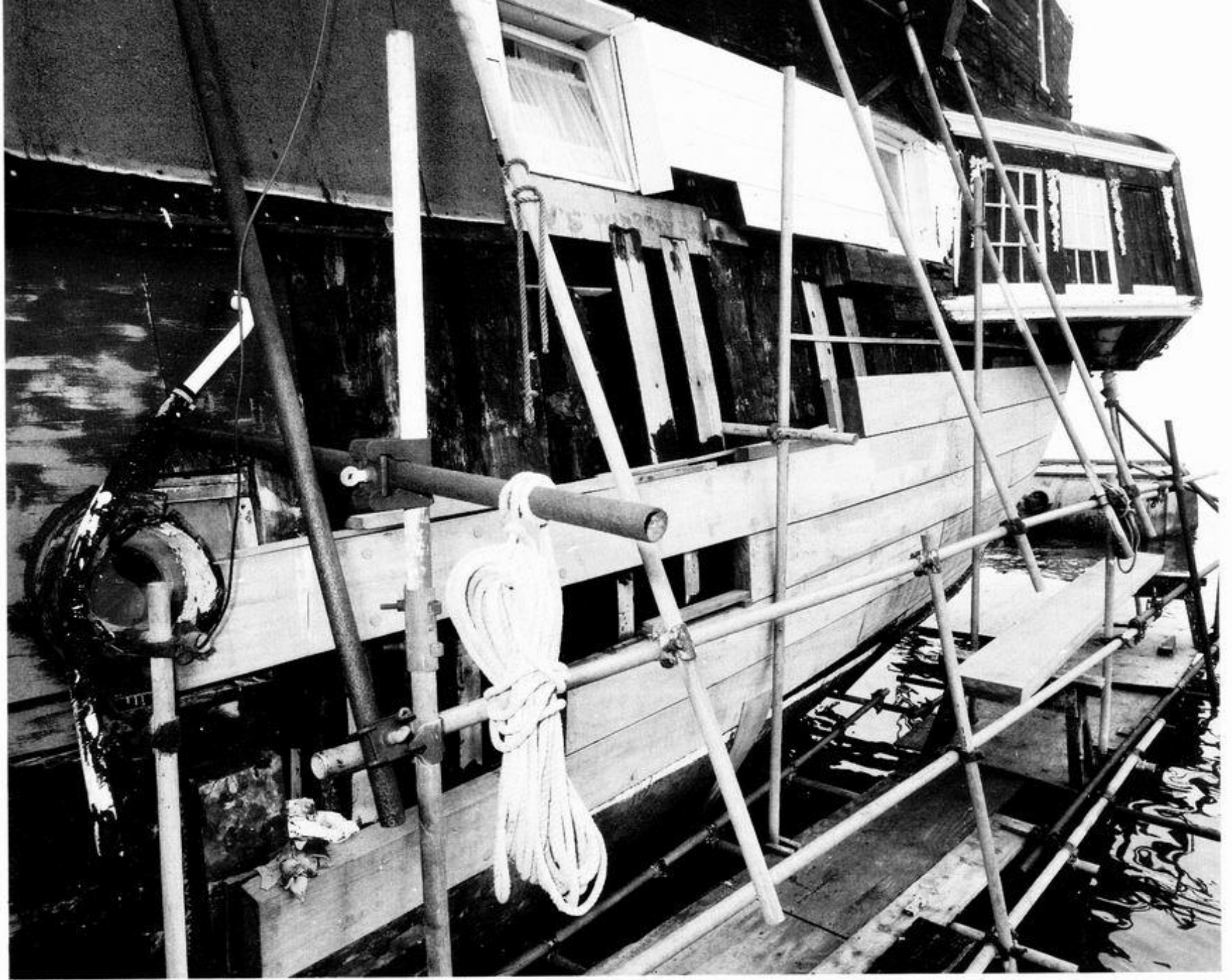
Above: Foudroyant. Port side, aft, showing the framing and gunport sill. The quarter gallery stool and lower finishing have been removed to allow restoration work to be carried out.
