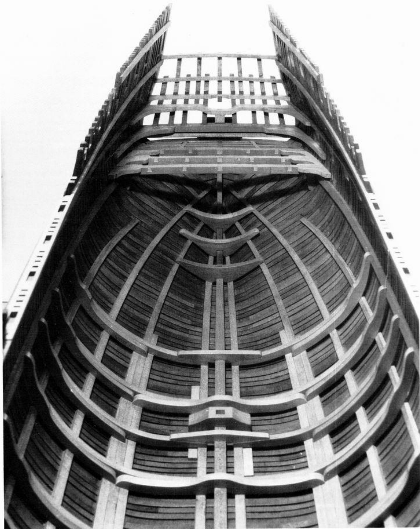
Egmont. The after body showing the keelson, sternson limberstrakes, thick stuff and deck clamps. The heavy internal frames are the floor and futtock riders. Also visible are the mainmast step and the crutches, one of which is adapted to form the mizzen step. The wing transom, the helm port transom and their associated transom knees can also be seen.
