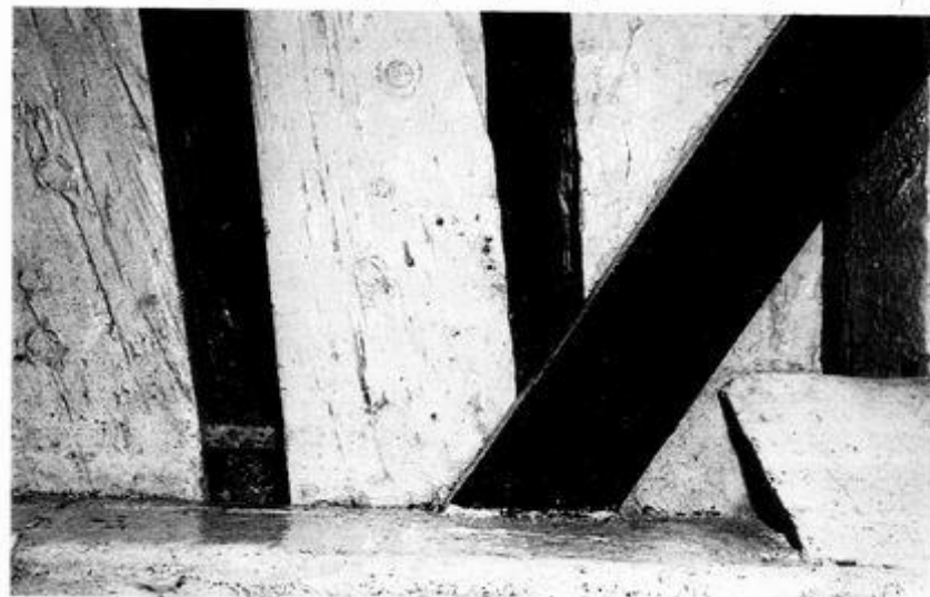
Unicorn. Close-up of timbers, starboard side, forward showing a square sectioned bolt driven horizontally between the frames holding them together and enhancing longitudinal strength. To the right is part of a diagonal iron rider plate.
