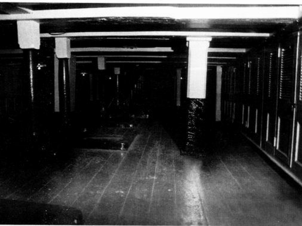
Left: Unicorn. The berthing deck, looking forward from the bulkhead that divided off the wardroom. The cabins shown here were usually used by the warrant officers and senior tradesmen such as the carpenter.
