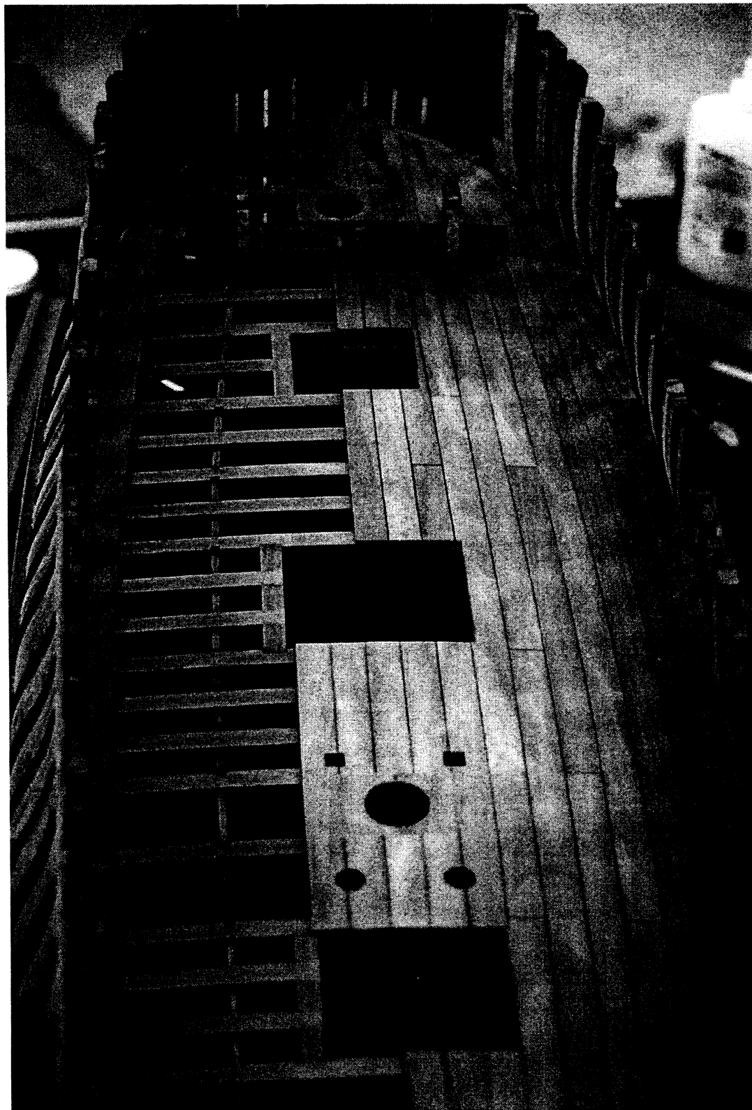
Figure 61. Deck planking on the starboard side of the model. Photo by G. Grieco.
