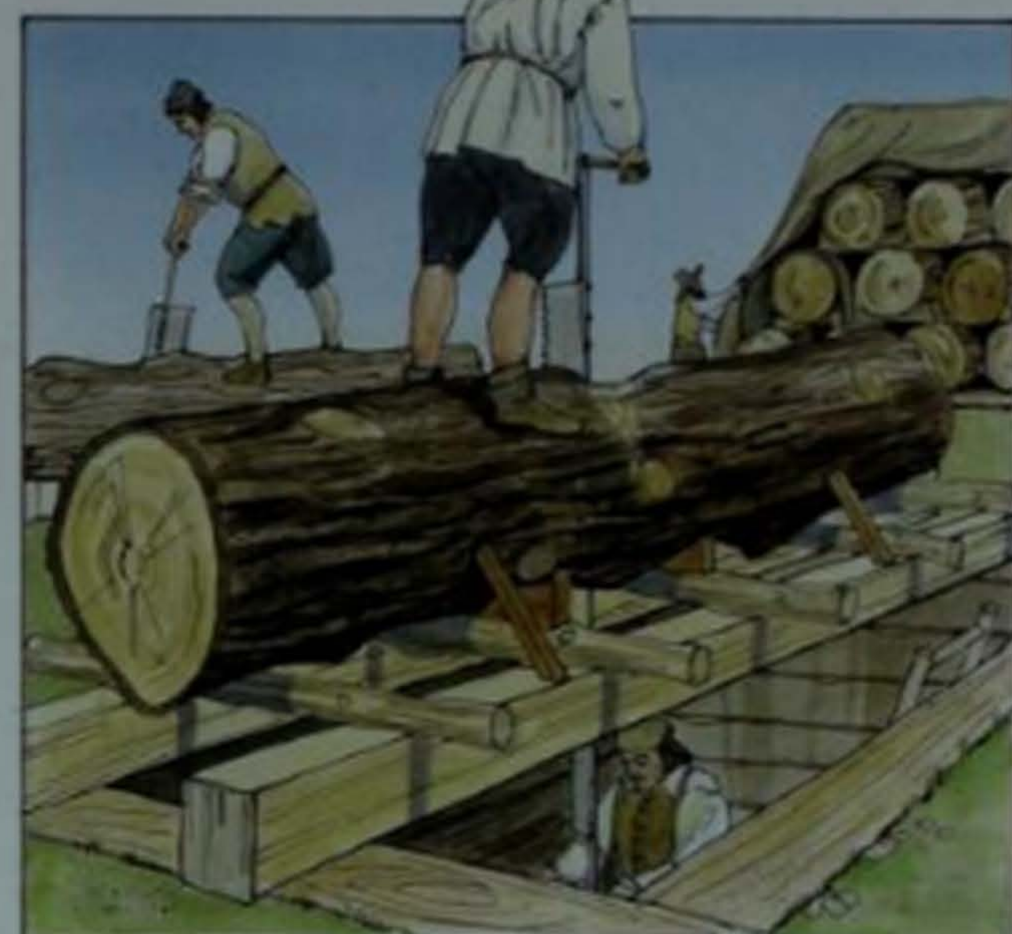
The busy scene (above) at a ship-building timber-yard shows the frames of a new galleon rising on the slipway beyond. Right: Rough timber being cut into square sections in the saw-pits. A long saw was used by two men, one standing on the timber and one in a hole (or pit) in the ground beneath. They pulled and pushed the saw up and down.
