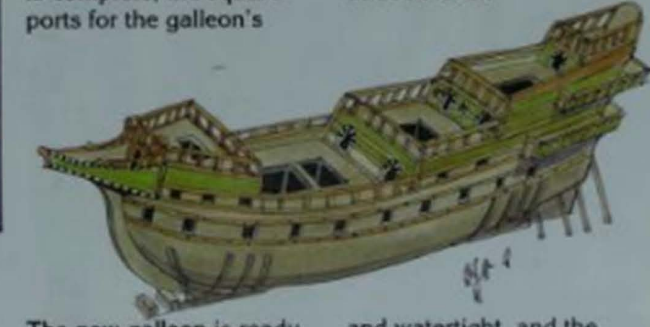
The new galleon is ready to be launched. All the seams are caulked
