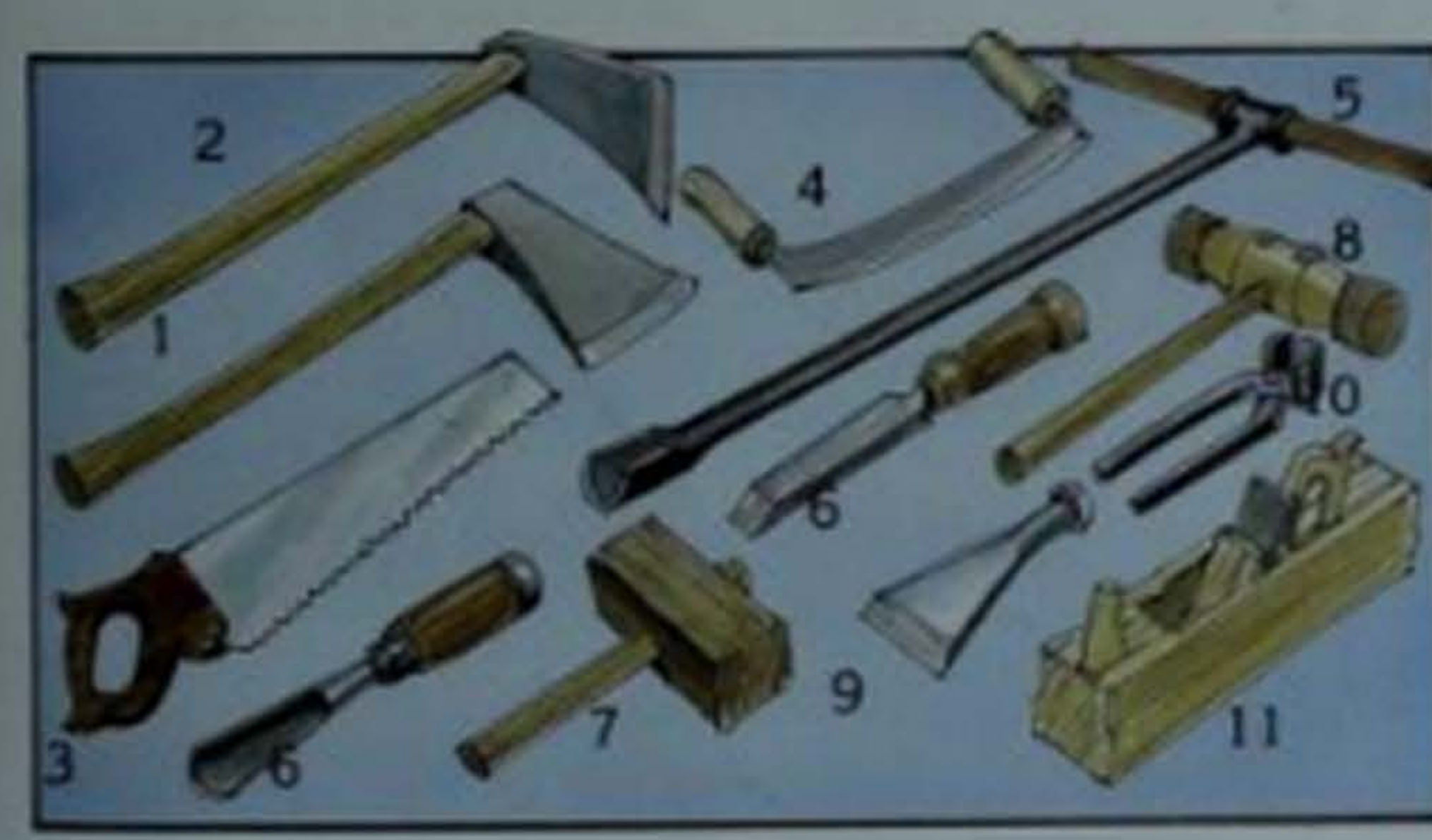
Carpenter's tools: (1) axe; (2) adze for smoothing surfaces; (3) saw; (4) draw-knife for rounding-off timber; (5) auger for boring holes; (6) chisels; (7) mallet; (8) caulking hammer; (9) caulking iron; (10) pincers; (11) plane.
