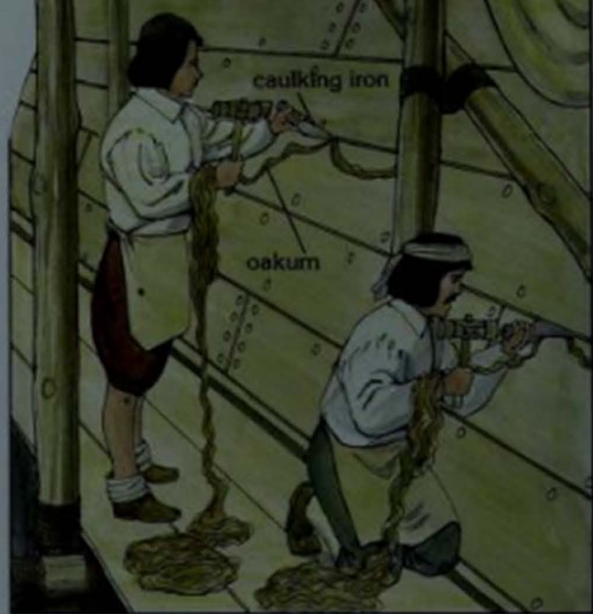
Caulkers at work (above), using hammers and sharp-edged
