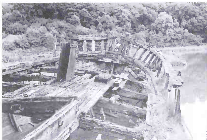
Fig 272. The decayed hull of the Millom Castle in the 1960s, looking forward from the main hatch. The steel tabernacle was a recent addition. (Author)
