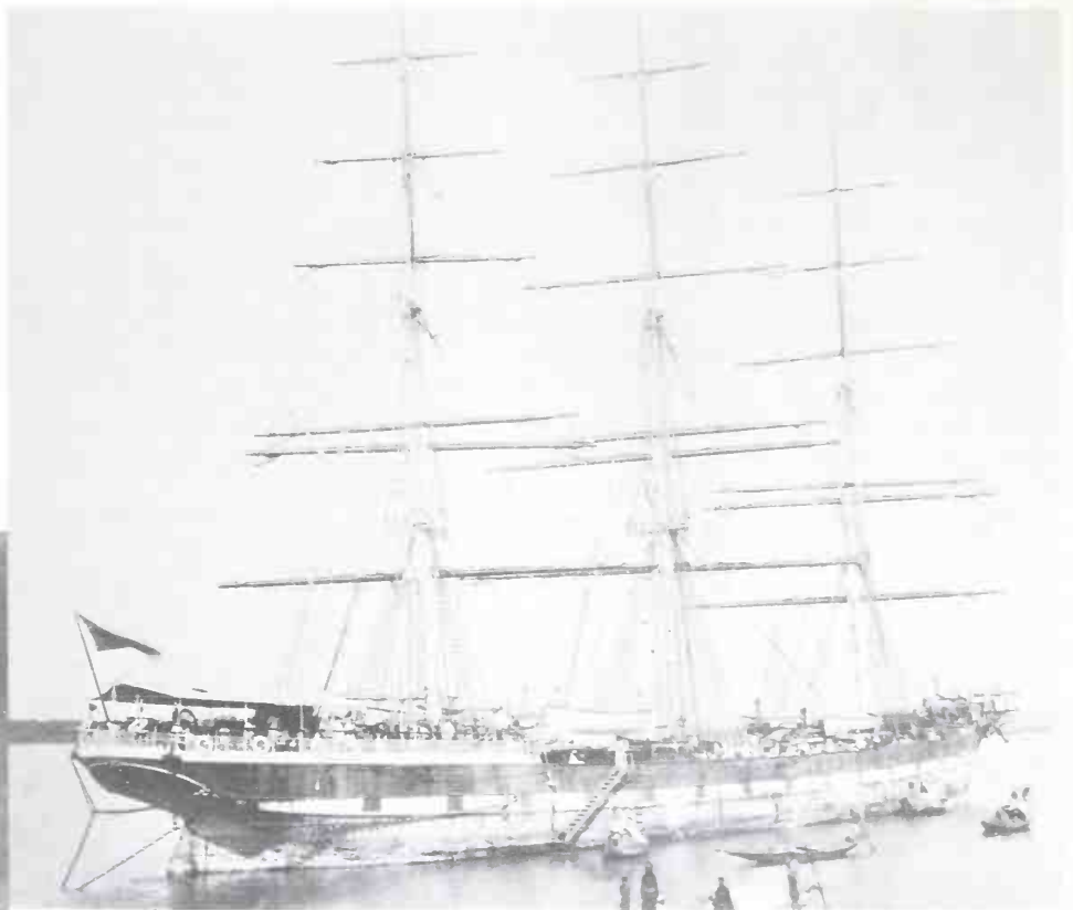
Fig 185. Another lofty ship was the Baron Colonsay, built in 1875 by J E Scott at Greenock. She was purchased from MacCunn by James Nourse in 1892 and renamed Lena, and it is with this name that she was photographed here at Calcutta. It is interesting that she had still retained skysail yards on each mast, but then Nourse did require his 'coolie ships' to be swift sailers. Her launch is described in the text at length. (Arthur D Edwardes)
