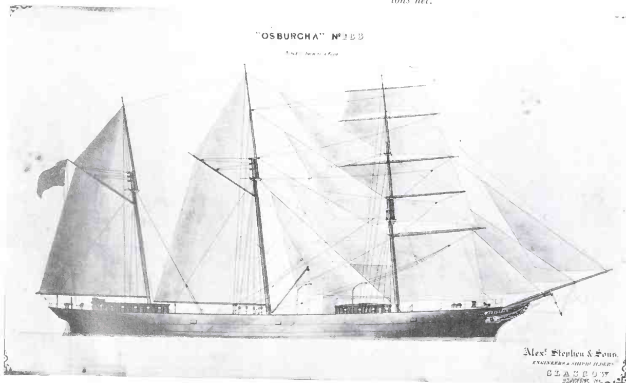
Fig 294. Osburgha. Sail and rigging plan photographed from original when in builder's possession. Built of iron at Glasgow in 1875 by A Stephen & Sons with dimensions of 146.7ft \times 26.1ft \times 13.0ft and 346 tons net.
