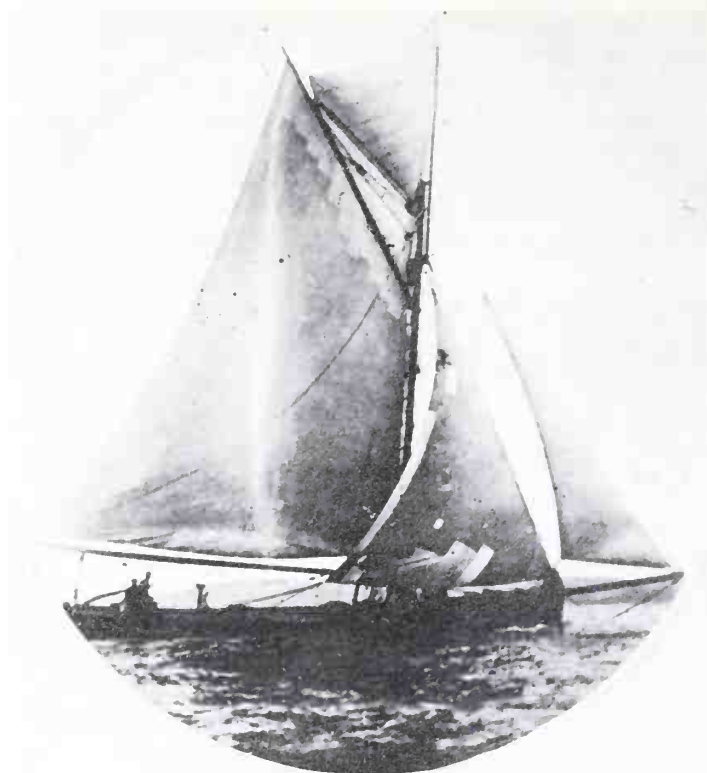
Fig 305. The boomie barge Lothair was built at Ipswich in 1872 with a tonnage of 108. She was owned at Rye. Her leeboard is just visible on her port side. Her fore yard is being used as a derrick, but her main topmast is missing and so is her jibboom. The inboard clasp for the latter is hinged open on the bowsprit, just above the fiddlehead. (David Clement Collection)
