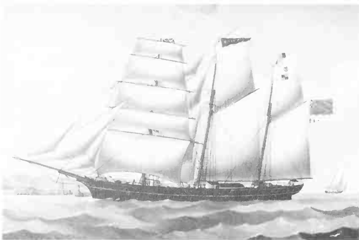
Fig 299. Oil painting of Unity inscribed 'Three-mast Brigantine "Unity" of Goole, Capn. G. Calvert, off Leghorn 1872' and it is signed 'L. Renault, Leghorn'. This barquentine was built of wood at Howden, River Humber, in 1871 by Banks with dimensions of 105.6ft × 24.3ft × 12.8ft and 179 tons. Lloyd's Register 1876 has her rig as schooner. The painting shows stunsail booms under the foreyard and large rectangular topsails on the main and mizzen with long head yards, and the hull is made to heel just enough to see the deck fittings. (Paul Mason Gallery)
