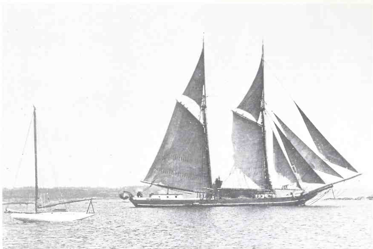
Fig 113. The American two-masted schooner Henrietta Simmons under sail in 1917. She was built in 1865 at Leesburg, New Jersey, with a tonnage of 228, and was assigned a 'full model' hull by the American Lloyd's Register. (Peabody Museum, Salem)
