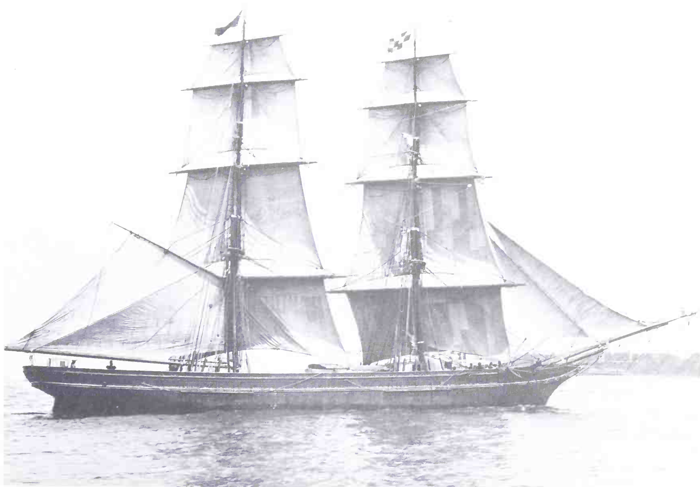
Fig 247. The Teazer close-hauled off Sandy Hook makes a dramatic picture with her single topsails, long trysail boom and fidded flying jibboom. Compare her with the sail plan in figure 246. (Peabody Museum, Salem)
