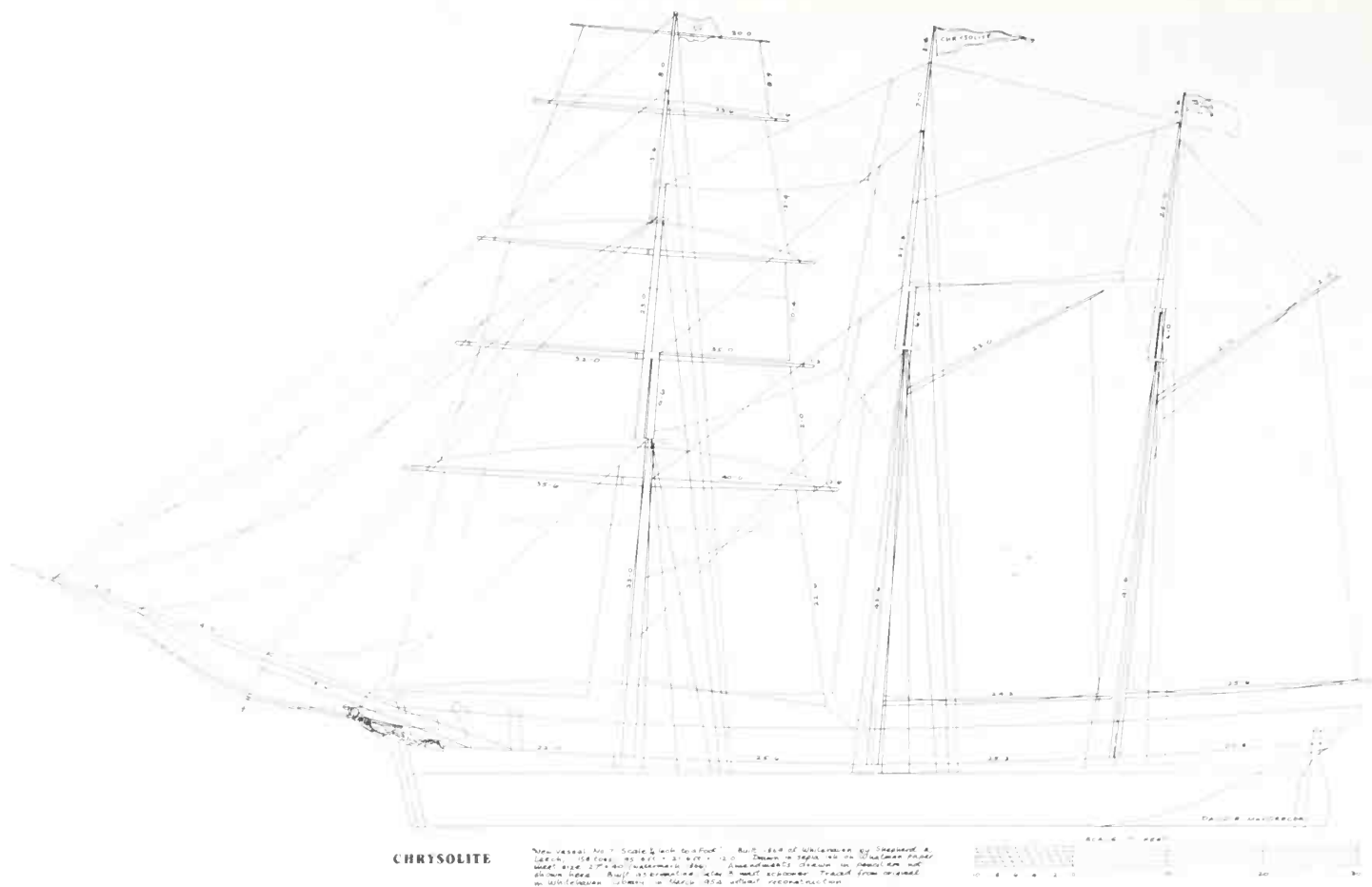
Fig 296. Chrysolite. Sail and standing rigging plan redrawn from tracing made of original in 1954. Built of wood at Whitehaven in 1869 by Shepherd & Leech with dimensions of 95.6ft \times 21.6ft \times 12.0ft and 158 tons. No reconstruction. Converted to 3-masted schooner 1887-91.
