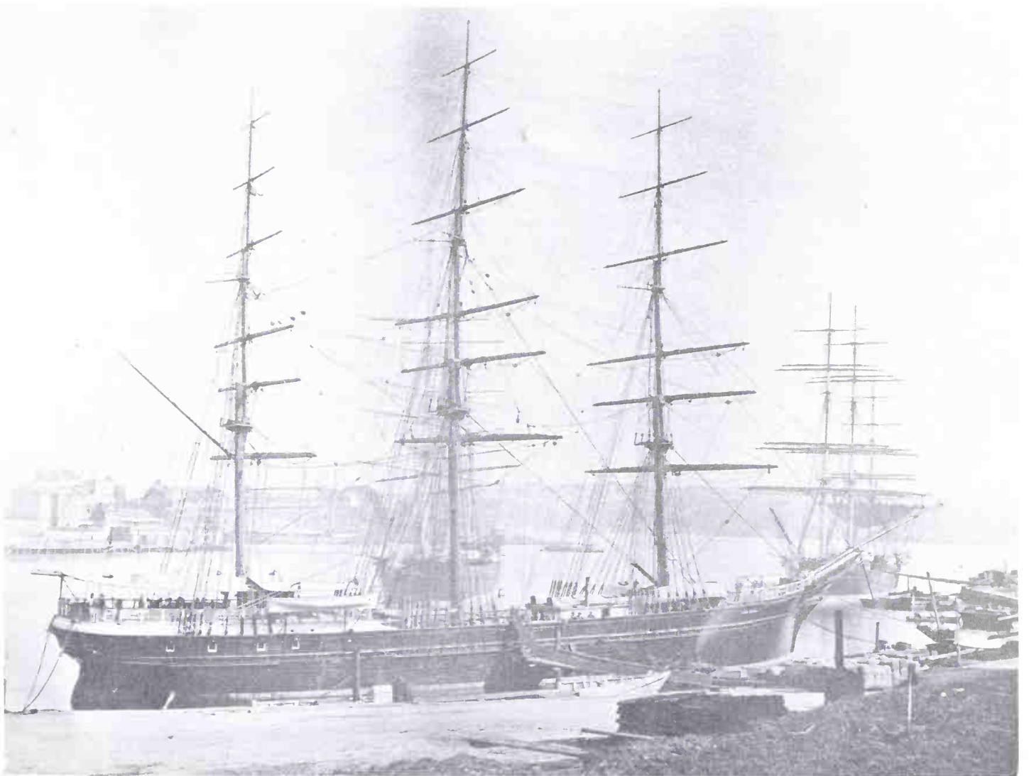
Fig 190. The John Duthie lying at Circular Quay, Sydney, set the style for many of the ships built by John Duthie, Sons & Co. She was built in 1864 with a tonnage of 1031 and a length of 196.0ft. Hoisting the upper topsails halfway-up the mast was considered to give a smarter appearance. (Cyril L Hume)
