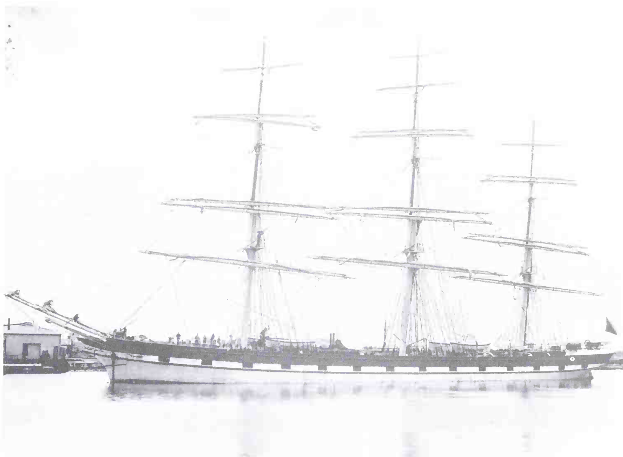
Fig 176 Barclay, Curle produced some magnificent iron clippers in the early seventies, but today it is difficult to imagine just how splendid they must have looked when newly completed. This photograph of Thessalus does give some idea of the appearance and the great spread of sail they carried on their long yards. The only thing to mar this picture is the shortened jibboom and missing dolphin striker. This photograph was taken by F Wear at Port Adelaide in December 1898 when she was sailing under the Swedish flag. (Anders Ericsson)
