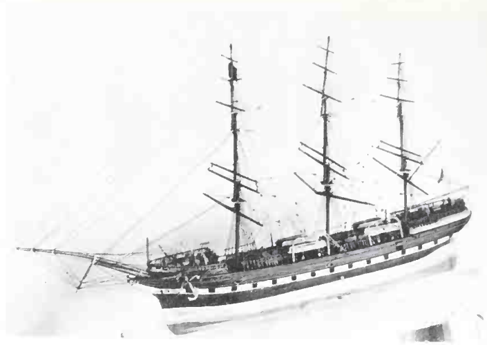
Fig 202. Model of England's Glory in the Sunderland Museum. She was built by William Pile in 1869. The placing of three boats with davits between the main- and foremasts is unusual, but the rest of the model portrays a large iron ship of this date very well. (Author)
