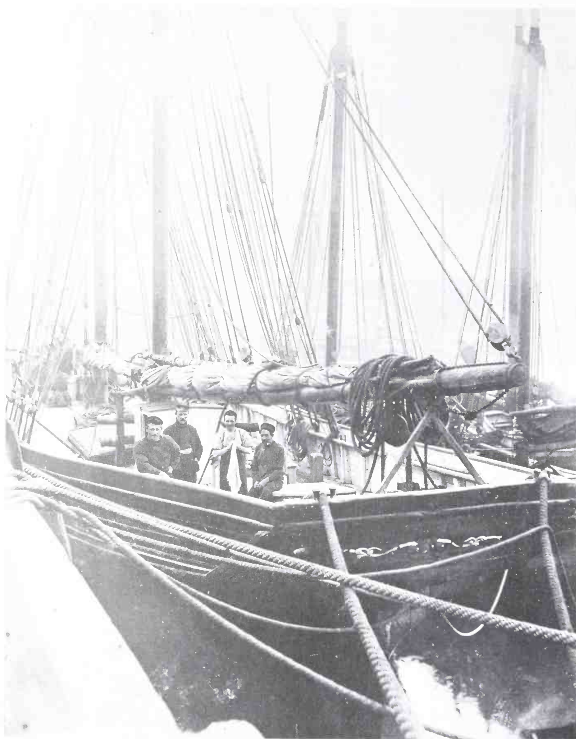
Fig 271. The stern of Amanda with her crew. She was built a year later than the Minnie, pictured under sail in figure 270, and by the same builder. They must have been almost sisters as the dimensions are virtually the same: net tonnage was 87 in each case; Amanda's dimensions were 82.7ft \times 21.3ft \times 10.1ft while Minnie's were 82.0ft \times 21.2ft \times 10.2ft. Both had square sterns. (R H Gillis Collection)
