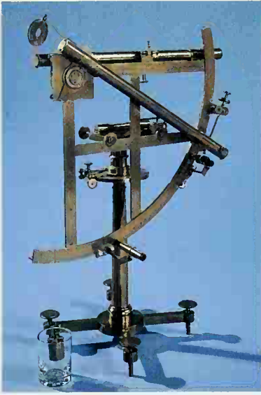
John Bird's 12 inch portable astronomical quadrant thought to be the one taken aboard Endeavour. It was used to measure the angular distance of the sun from the zenith (the point immediately overhead), from which the accurate latitude and longitude of the observer could be obtained.
