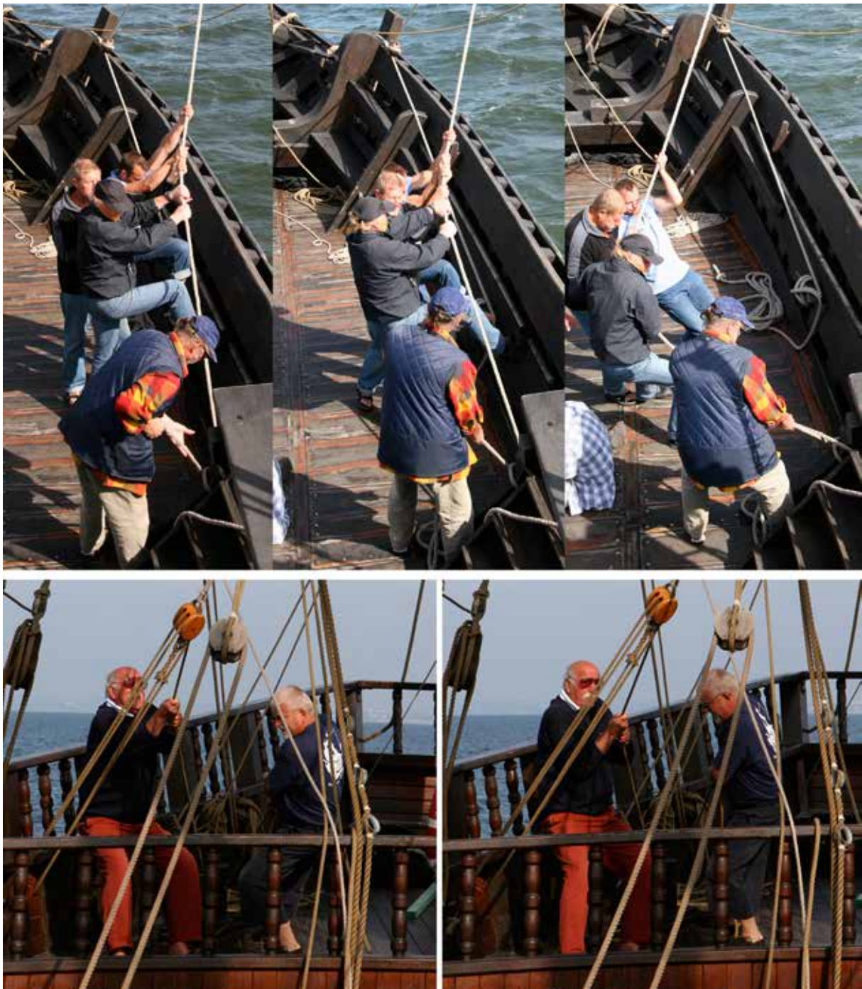
Fig. 23. Experimental sailing trials with the KIELER HANSEKOGGE and the multi-masted LISA VON LÜBECK as a rebuild of a 15 th century ship allow comparison and indicate the simplification of the work with the running rigging through the invention of blocks and tackle. above) Hauling the sheet of the KIELER HANSEKOGGE, below) Hauling the sheet of the fore sail of the LISA VON LÜBECK.
