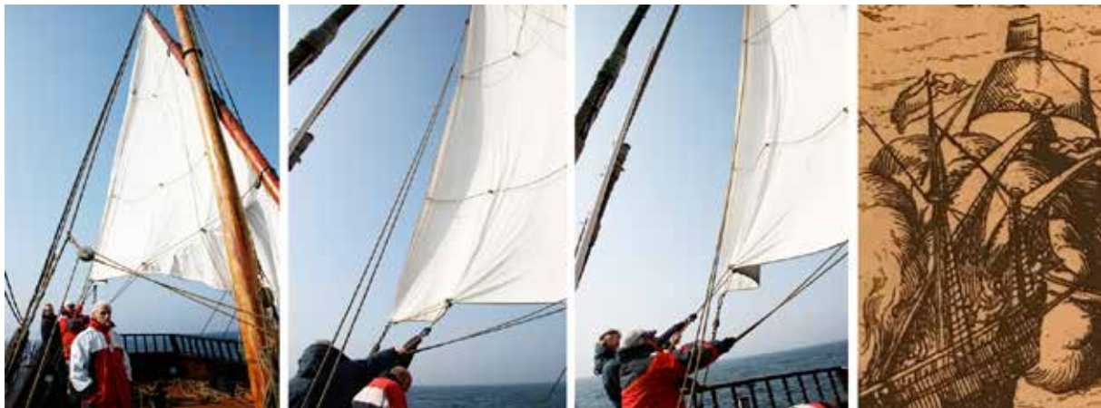
Fig. 14. Left: Sailing trials with the LISA VON LÜBECK demonstrate the usage of the lateen only during tacking windwards (Photos: M.-J. Springmann). Right: the same could be interpreted from a copper engraving of the Admiral ship MARS from the sea disaster of 31 st May 1569.
