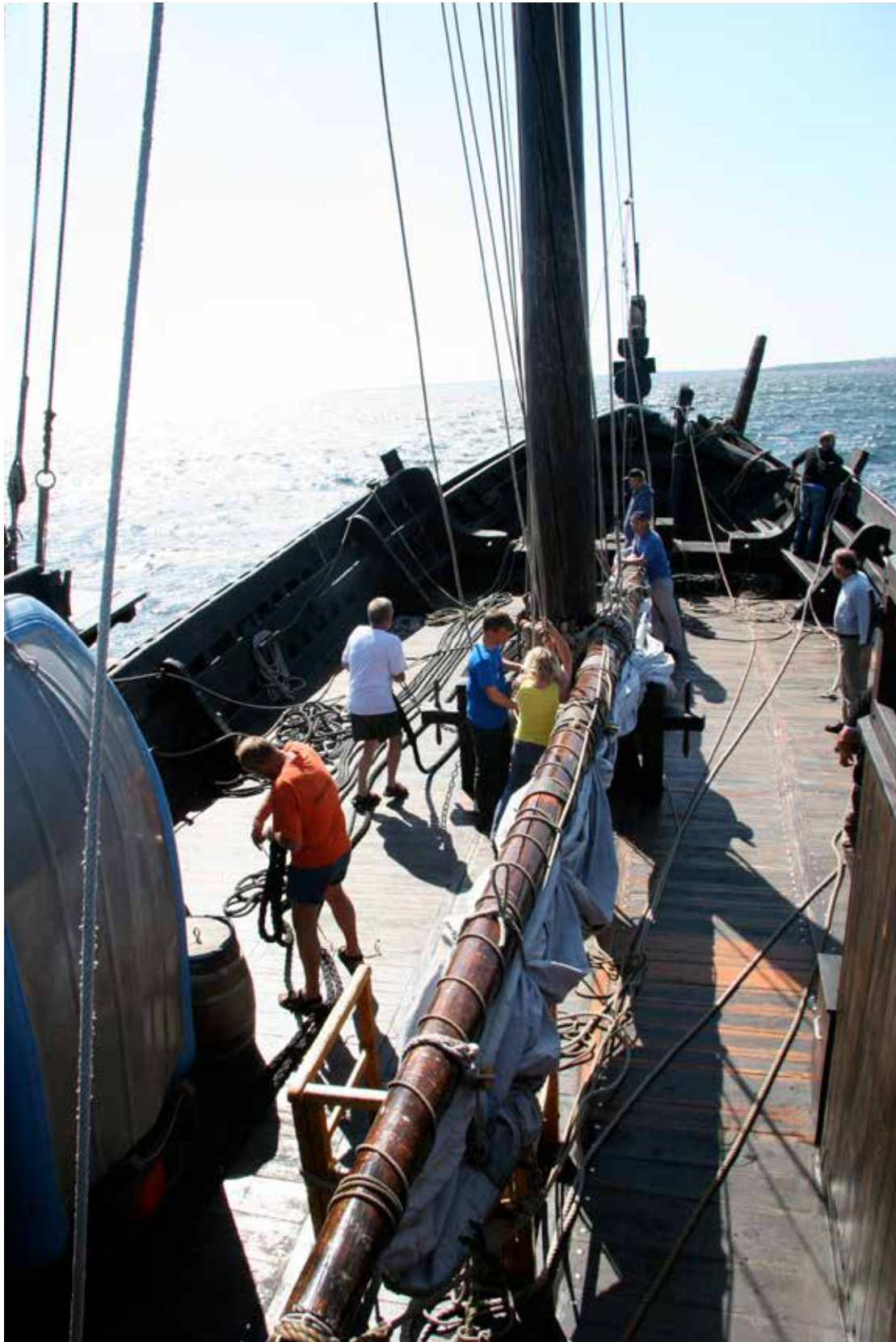
Fig. 18. The yards aboard vessels like the Bremen type from 1380 could be lowered in the way demonstrated in this photo of the replica of the ship KIELER HANSEKOGGE.
