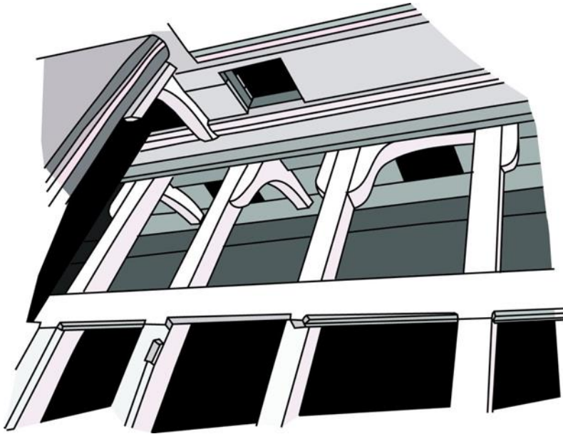
Fig. 22: Illustration of the upper-deck and the edge rail of the quarter-deck. The only two visible deck planks are the waterway and the binding strake, which is rabbeted to receive the hatches. Ditta 2014.
