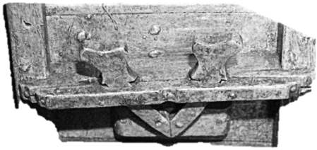
Fig. 24: detail of a “finger and thumb” fashion kevel. Ditta 2014.
