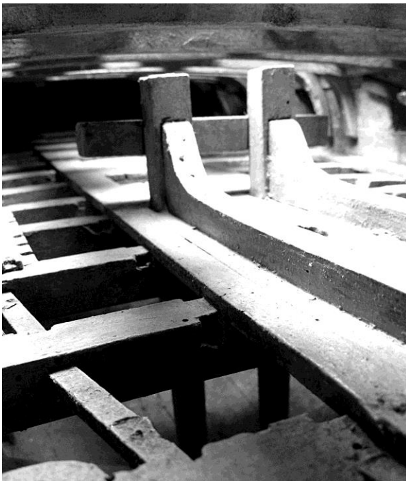
Fig. 21: Detail of the riding bitts. Ditta 2014.
