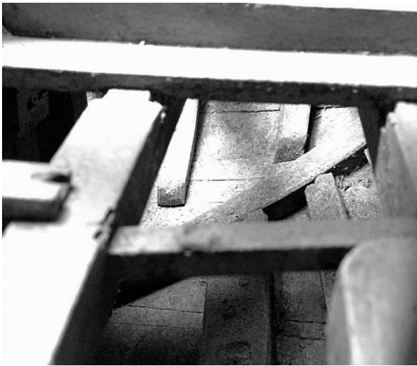
Fig. 17: On the background, detail of the port-side compass timber laid diagonally at the bow. Ditta 2013.
