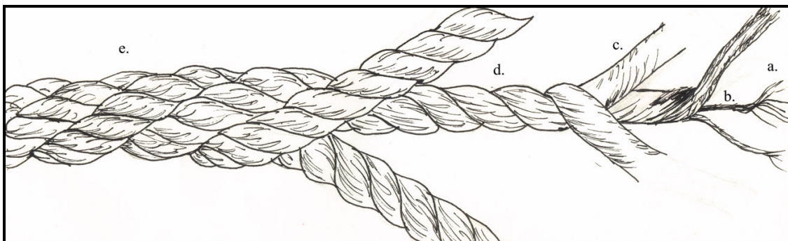
Figure 8. Diagram of an s-twisted cable: (a.) z-twisted fiber, (b.) z-twisted yarn, (c.) s-twisted strand, (d.) z-twisted hawser, (e.) s-twisted cable. Drawn by J. McCaskill.
