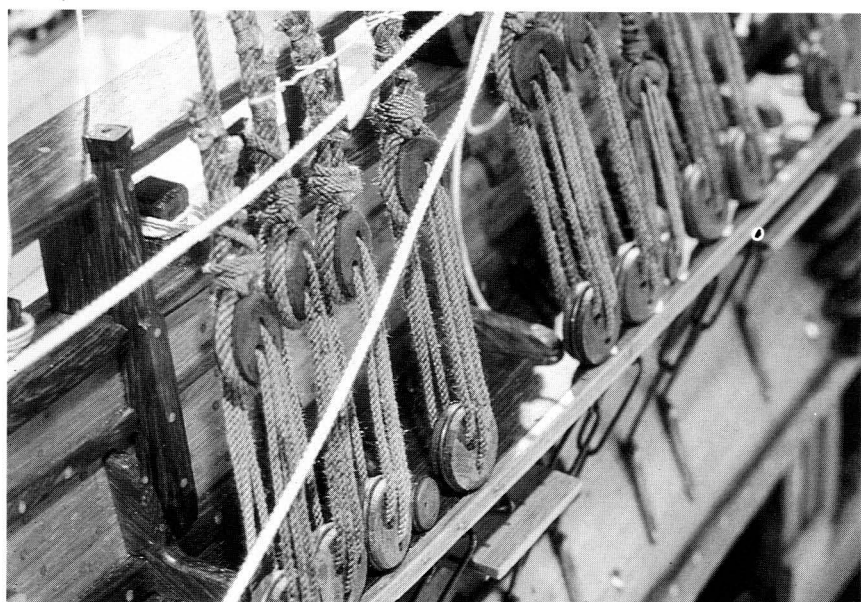
14. The main channel, starboard showing shrouds, deadeyes and lanyards.
