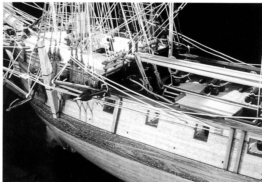
12. The model's forward waist. Note that the modeller has placed spare spars along the centreline of the waist and has not shown skid beams and boats. The drawings show Pandora equipped with gang boards and skid beams for boat stowage and in this case spare spars would have been stowed between the boats and on the channels.
