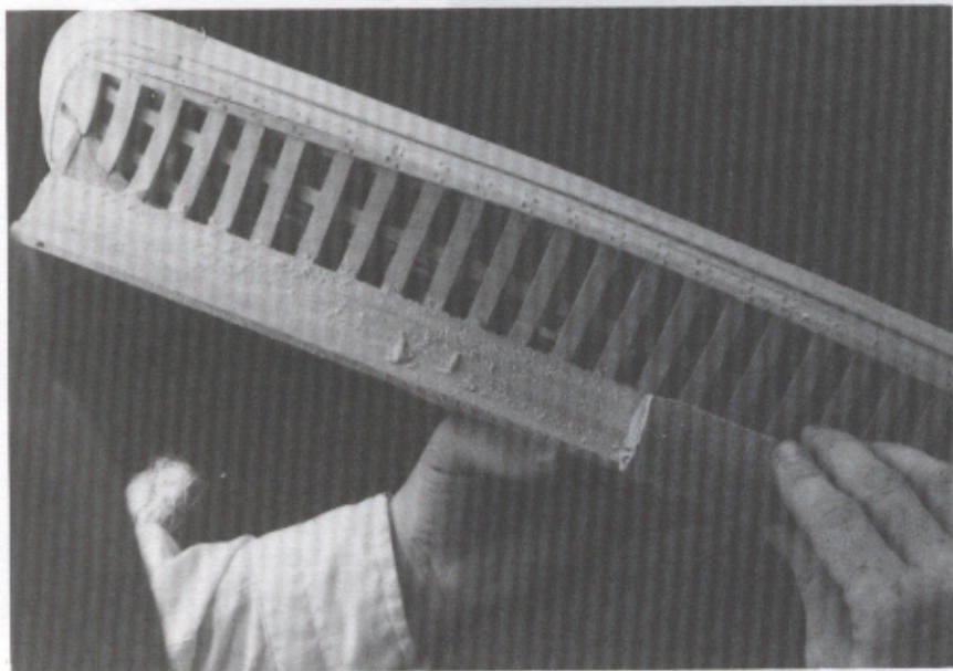
62. Final stage of planking is sanding tree-nails flush—starting with No. 80 paper and finishing with No. 220.
