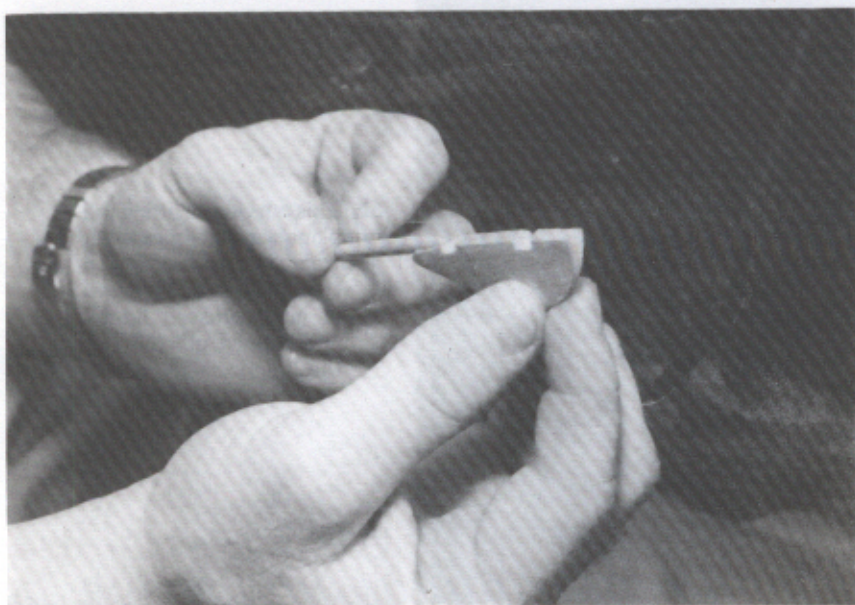
64. Now the rudder is completed, the gudgeon and pintles fitted and the rudder hung on the sternpost.
