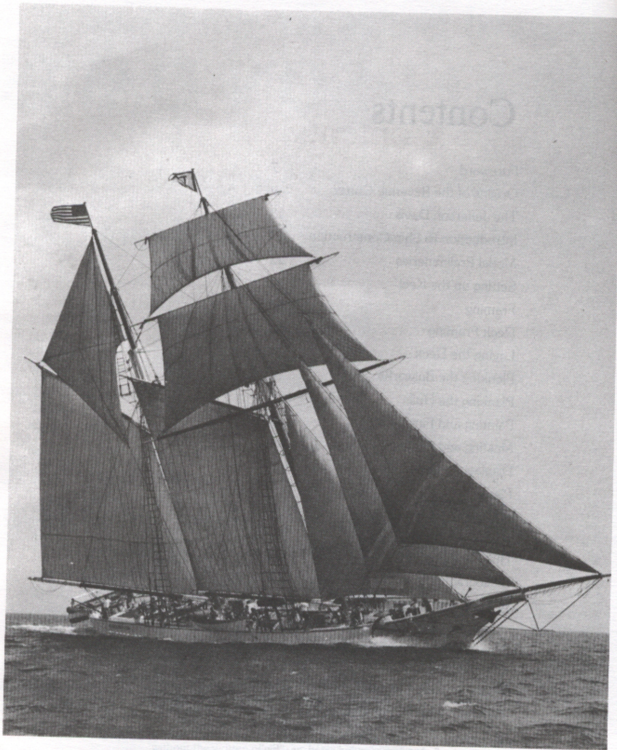
The power and beauty of the Baltimore Clipper topsail schooner design is clearly dramatized in the photograph. This is Capt. Robert Douglas's Shenandoah , a modern-day Campbell class cutter which sails out of Vineyard Haven, Mass. Close-hauled on the port tack she is showing a good turn of speed in a gentle breeze. Norman Fortier Photograph.
