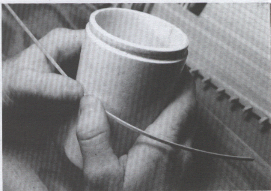
21. After soaking in boiling water for a few minutes wood strips can be formed to curves around a suitable form.
