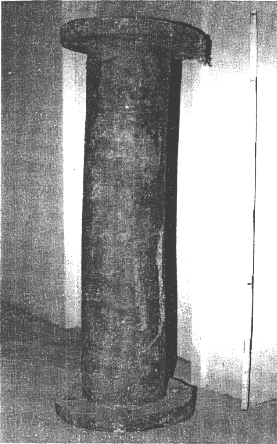
Figure 15. A corps de fonte from a French Royal Pump. The cast bronze section was fastened between two wooden tubes. A bronze piston valve worked within it. (Photo by the author)
