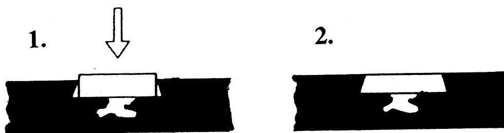
Fig. 9. The application of a bronze patch to an undercut bed over a faulty surface. (Drawing by the author)
