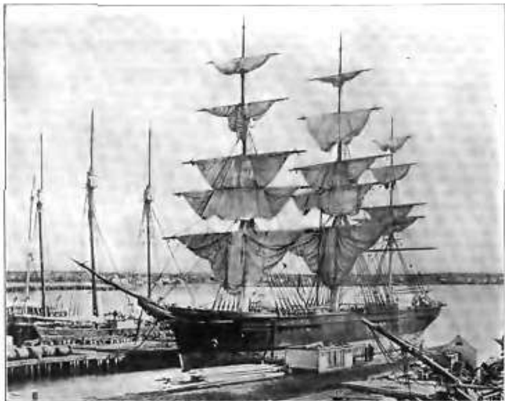
[275] SHIP "SIREN," OF SALEM, 1064 TONS, BUILT AT MEDFORD IN 1851. From a photograph taken at New Bedford.
