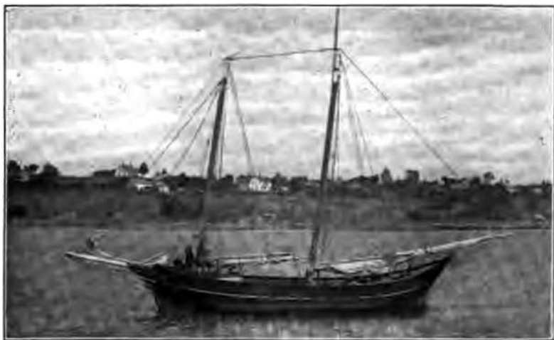
[177] PINKY "MAINE," 24 TONS, BUILT AT ESSEX, MASS., IN 1845. A type of small vessel once in general use along the New England coast both for freighting and fishing. From a photograph taken in Belfast, Me., harbor.
