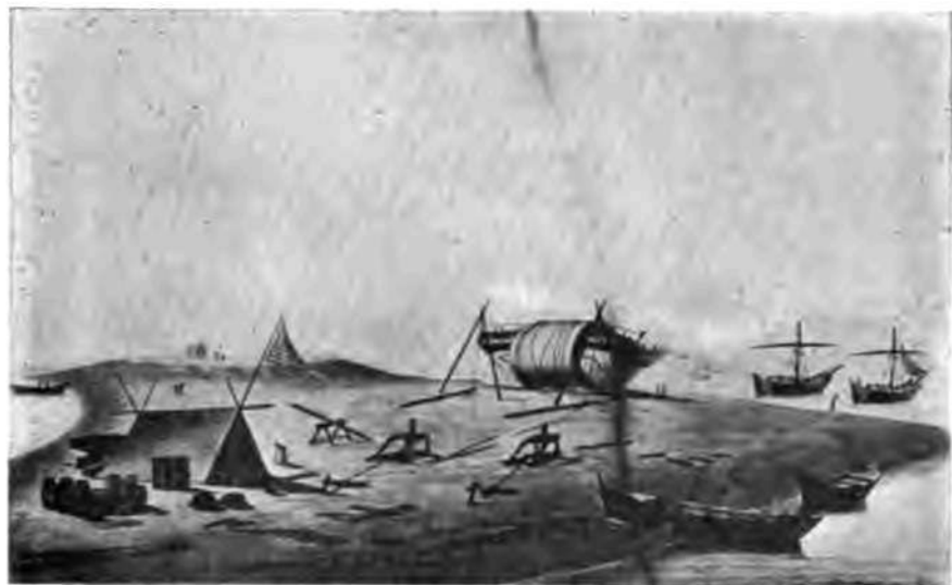
[88] BRIG "EUNICE" OF SALEM, 145 TONS, BUILT AT BARNSTABLE IN 1803. From a water-color by Anton Roux, showing device for launching the vessel after cleaning its bottom at St. Paul Island in 1817.
