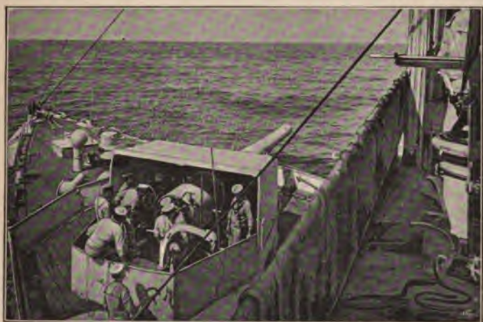
9.2" 22-TON BREECH-LOADING GUN AS MOUNTED IN BOW OF H.M.S. "BLENHEIM."
