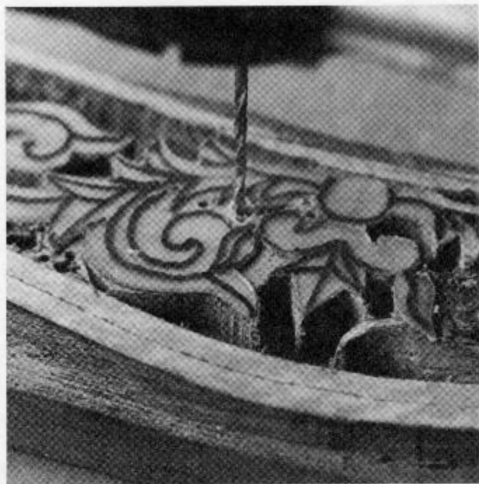
Fig. 10-29. Drilling out the wood in preparation for carving a scroll (Courtesy of David Stevens).
