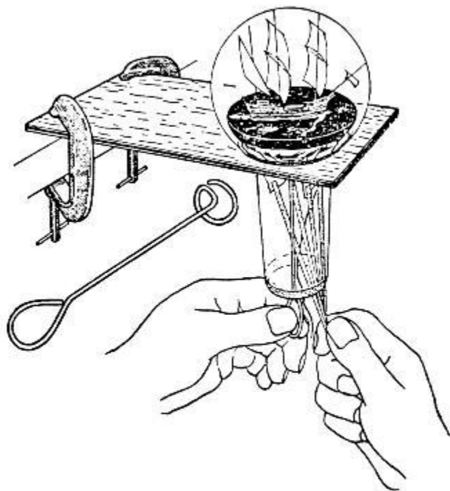
Fig. 6-8. Removing the turning mechanism with the aid of the holding device. The device is made from an old metal coat hanger (Courtesy of Model and Allied Publications, Argus Books).
