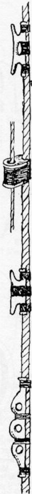
Fig. 14-5. Attaching cleats and fairleads to the shrouds (Courtesy of Northshore Deadeyes, Ltd.).
