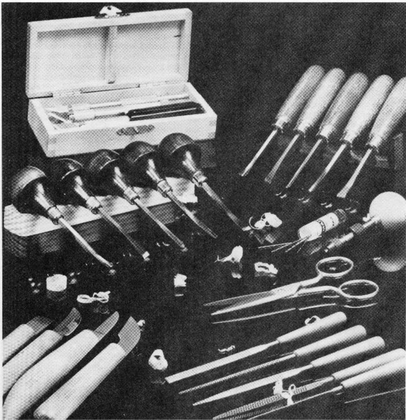
Fig. 3-4. A collection of carving tools, gouges, and rasps. A pin vise and drill bits are shown center right (Photo courtesy of Mascot Tools).
