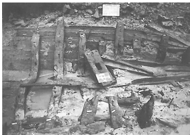
Figure 4-30: Disarticulate mast step in stern section of the Bremen Teerhof wreck (Brandt, 1979 p. 325)
