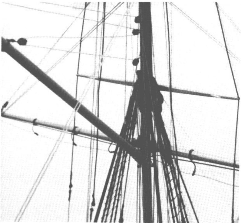
Top The fore side of the mast at the doubling; the spreader and crossjack yard are prominent.
