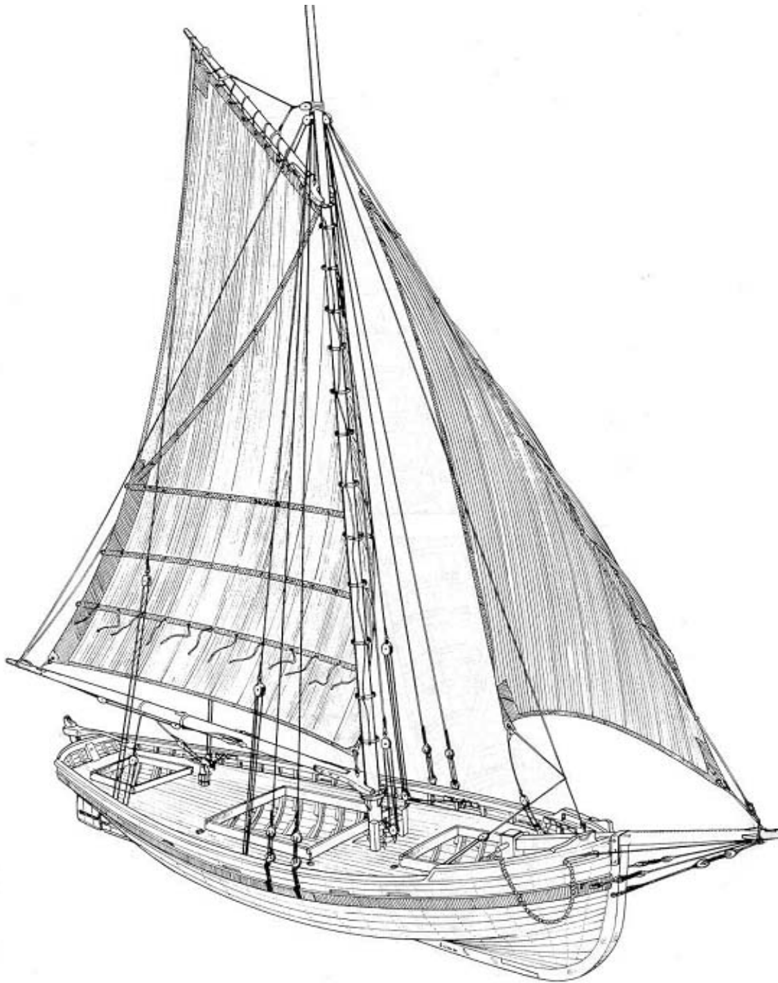
Figure 38. Reconstruction of the Malcolm Boat with a Gaff Rig (drawing by William R. Judd, courtesy of SCIAA).
