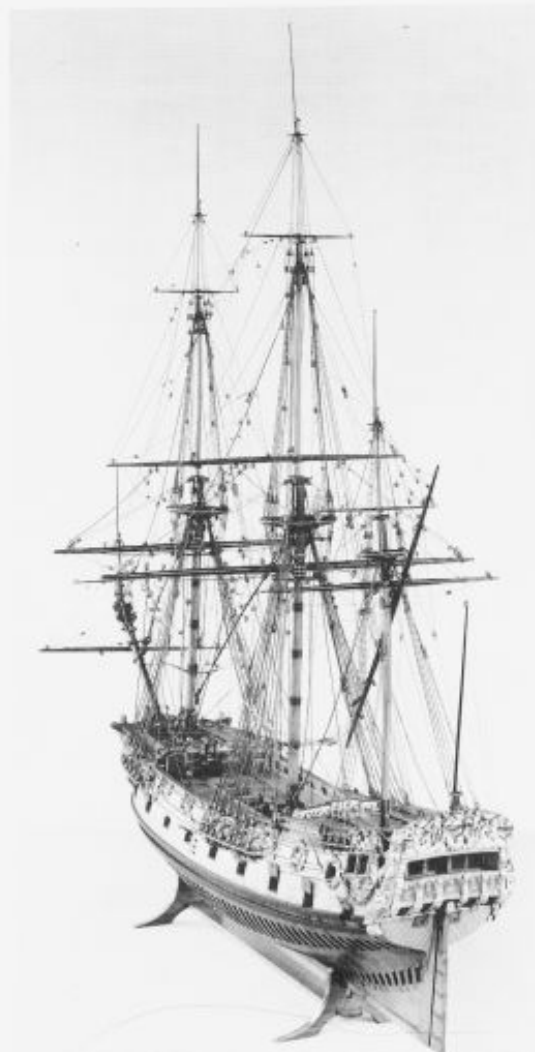
Although this model of a 50-gun ship of about 1685 cannot be identified with a particular ship, the rigging is believed to be almost entirely original, so is a reliable source of information on even the most minute aspects of top hamper during this period. (NMM: B9914)
